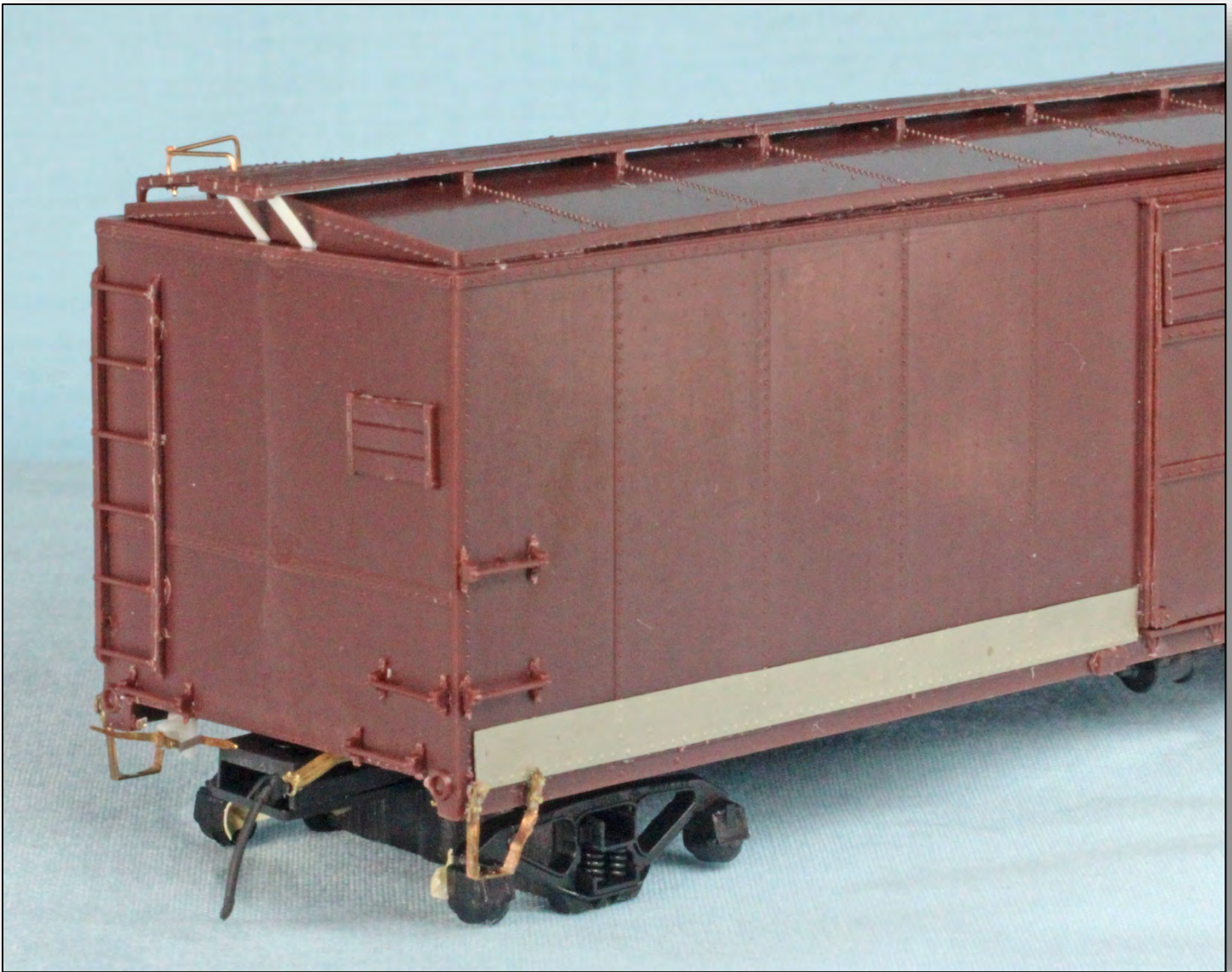
Brake end view of car with full length patch panel showing Carmer uncoupling lever.
