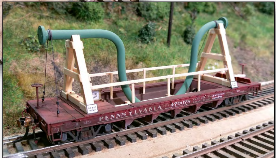
Tie-down cable attachment points are different at each end due to the load's asymmetry.
