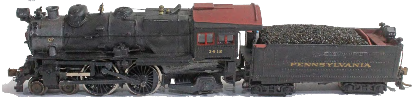
Francis Treves modeled E6s #3412 in N-scale as it looked in the late 1940's. He kitbashed the mechanism from a Mini-Trix K4s, shortening the chassis and removing a driver. He shortened the pilot truck and modified the length of a Shapeways tender. He kitbashed the boiler from the K4s, added a smokebox door from a Kato LIs, added a Shapeways cab and a sand dome. The firebox came from the LIs. Added details included marker lights, working headlights from an LIs conversion kit, wire piping, brake shoes, pewter air pump, bell, generator, and whistle deflector. Paint is Floquil acrylic and decals are by Microscale.
