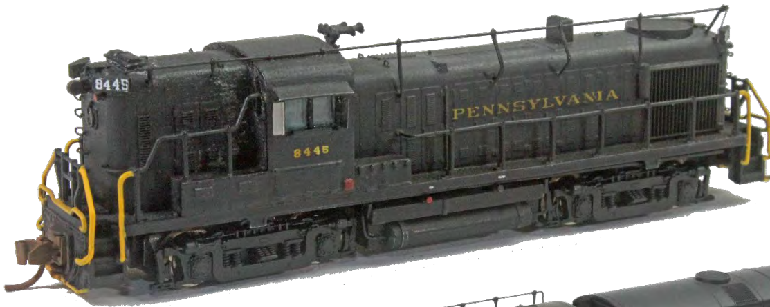
Francis Trevey modeled PRR's only hammerhead RS-3 in N-scale as it looked in the 1950's. He started with a Kato RS-3 and made multiple prototype-specific modifications.
