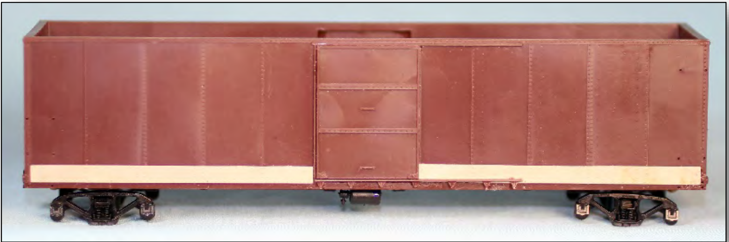
The long patch panels glued to the side of the car.
