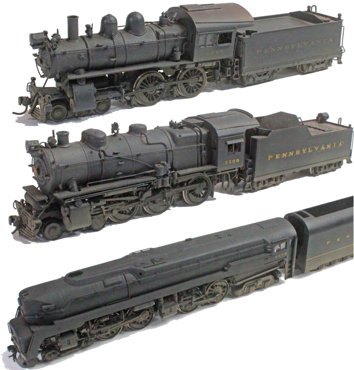
David Wilson brought three HO-scale steam locomotives to the Model Room this year. From the top are D16SB #1046, G5s #3109, and T1 #5544. They are painted with Floquil Brunswick green, Floquil Zinc Chromate primer, Floquil earth, Floquil grimy black, and Wilson's Modelworks decals. The T1 has Microsoft stripes and keystone.
