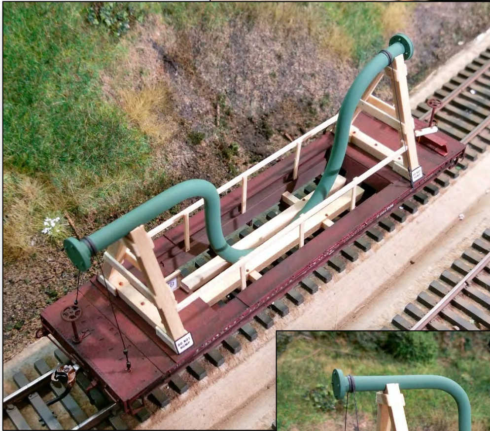
Tie-down cable attachment points are different at each end due to the load's asymmetry.
