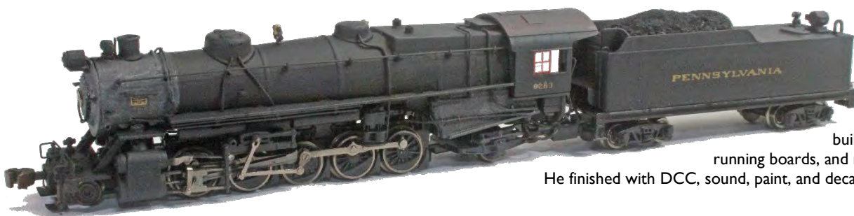
Francis Treves modeled E6s #3412 in N-scale as it looked in the late 1940's. He kitbashed the mechanism from a Mini-Trix K4s, shortening the chassis and removing a driver. He shortened the pilot truck and modified the length of a Shapeways tender. He kitbashed the boiler from the K4s, added a smokebox door from a Kato LIs, added a Shapeways cab and a sand dome. The firebox came from the LIs. Added details included marker lights, working headlights from an LIs conversion kit, wire piping, brake shoes, pewter air pump, bell, generator, and whistle deflector. Paint is Floquil acrylic and decals are by Microscale.
