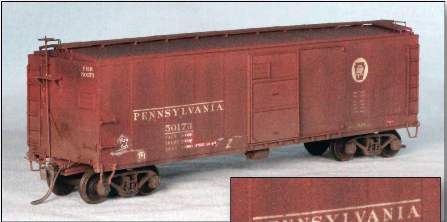
The kit after painting, decals, and weathering. The close up shows the re-weigh and lubrication dates masked to look repainted.
