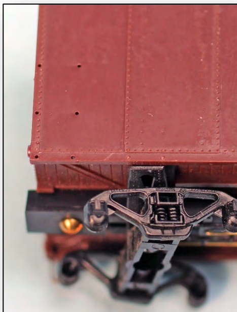
Holes drilled in car side for pins and brass wire pins placed for sill steps.
