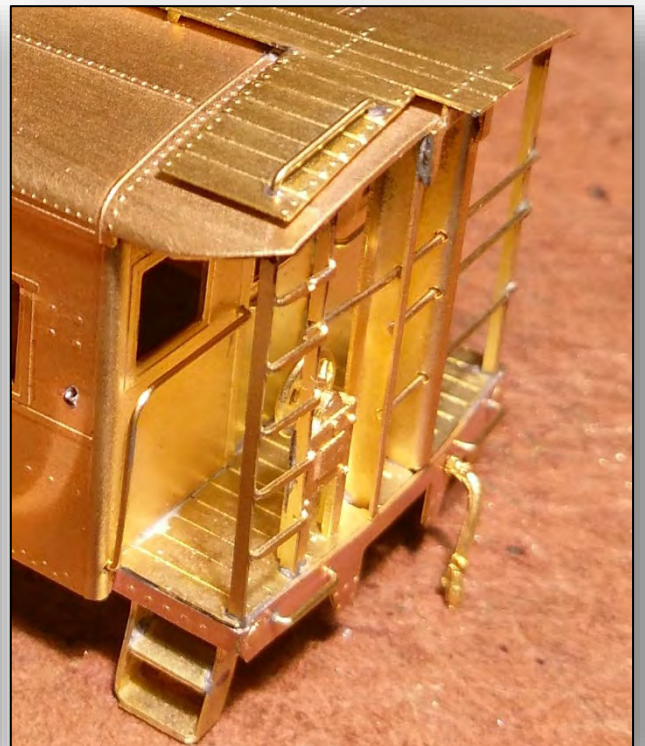
End views of as-purchased model illustrate problems: three end handrails running through the collision posts, sharp roof corners and missing details.
