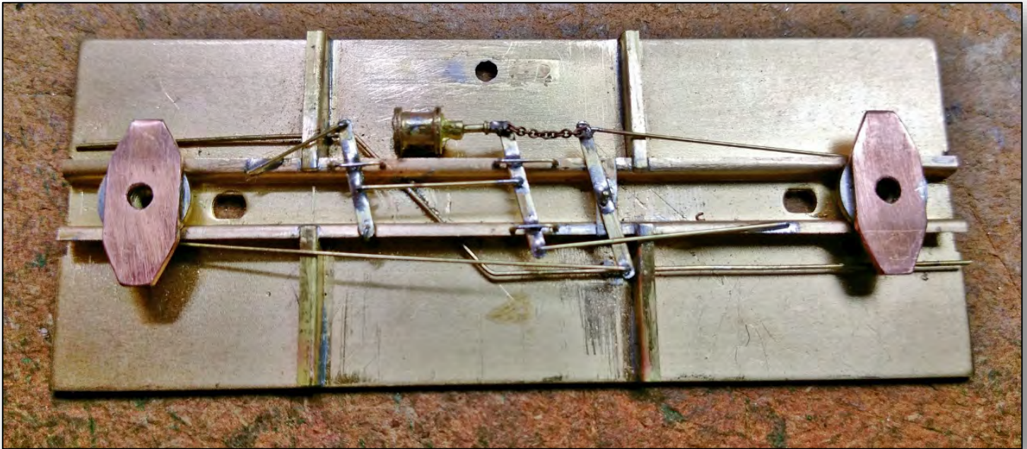
▲ Bolster plates, cross bearers, trainline and mechanical brake components added to underframe. ▼ Completed underframe.
