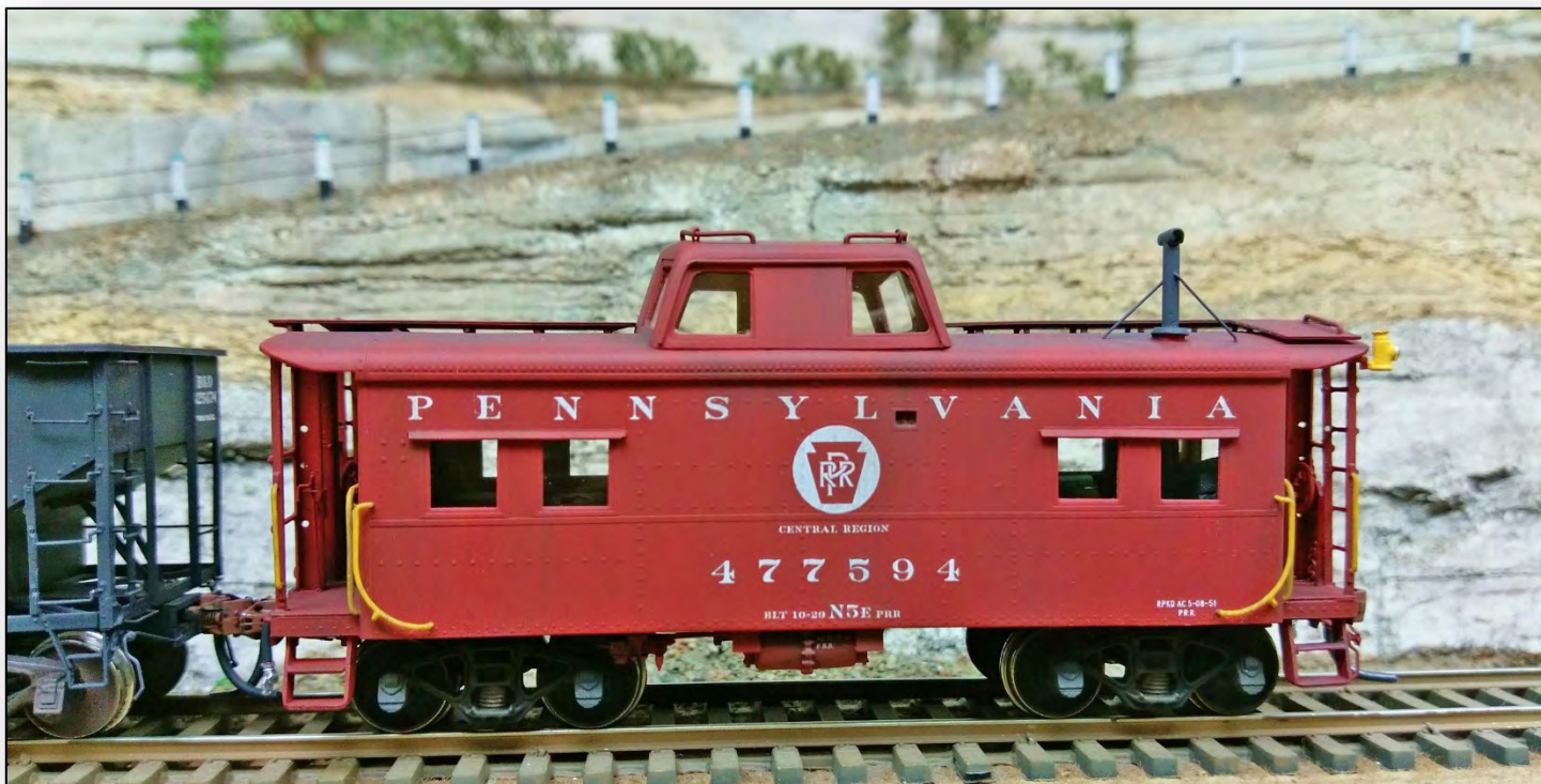
Broadside view illustrating proper location and spacing of the lettering.
