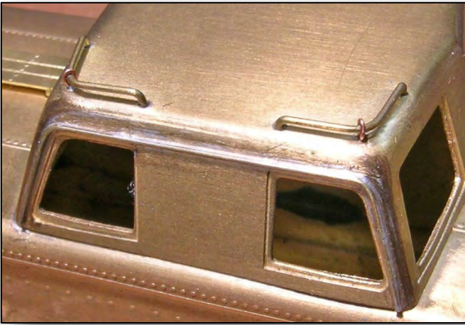
Cupola detail showing replaced side rain gutters and added third legs to original grab irons.
