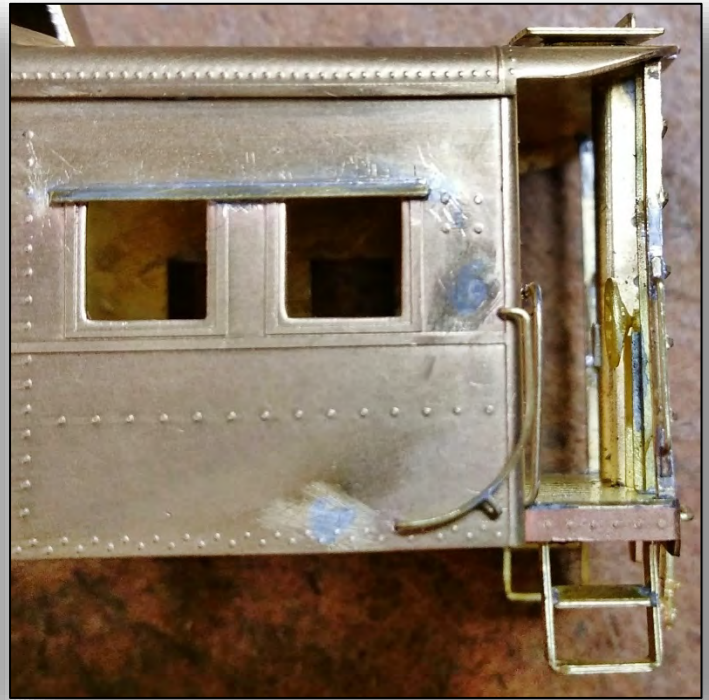
Left photo shows corner grab in place with temporary spacer, ready to solder. Backing piece for lavatory vent can be seen inside car at right center. Right photo shows finished corner grab with third support and original holes filled.
