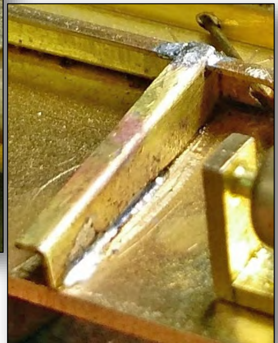
Cross bearer tack-soldered to floor near outer end at left, heat being reapplied further along part at center, and finished joint resulting from subsequent wicking at right.
