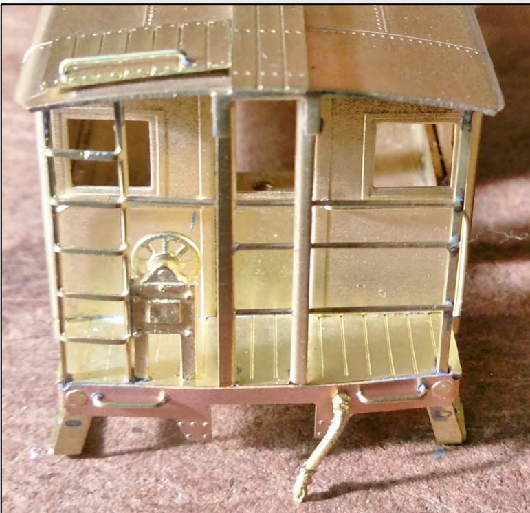
End views of as-purchased model illustrate problems: three end handrails running through the collision posts, sharp roof corners and missing details.
