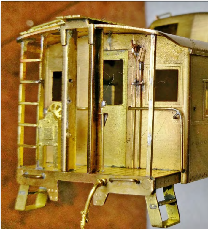
Rear end of car at left, front end at right. Added details include: retainer and whistle valves with air lines on end sheets; third (center) support legs on end "L" grabs; brake valves and lines attached to right hand collision posts with small brackets.
