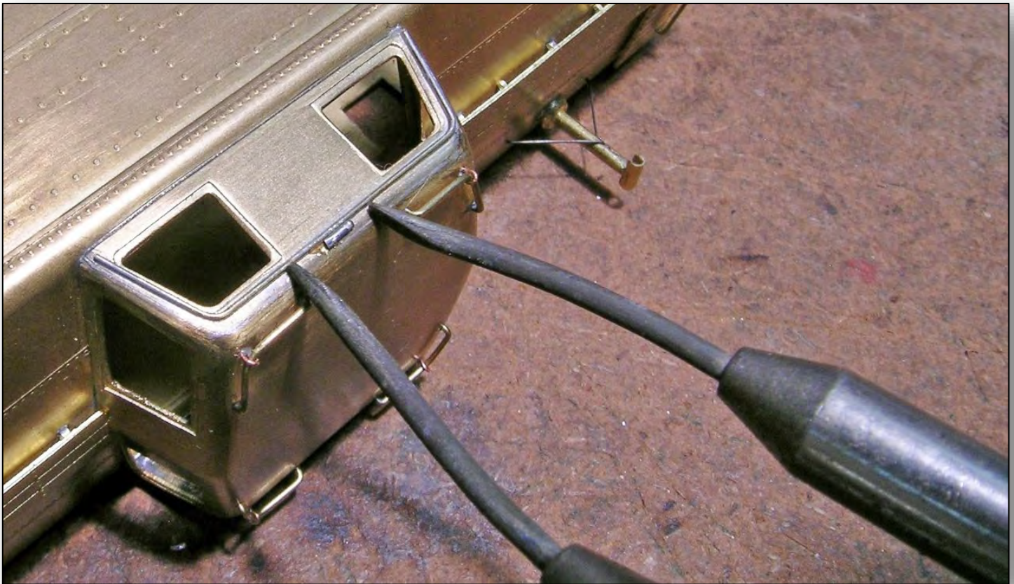
Soldering technique where the tweezers cannot reach inside the area desired. Tweezers are held against the base surface straddling the area to be heated. Short length of solder wire is stuck in place at spot desired with flux, ready for heat to be applied.
