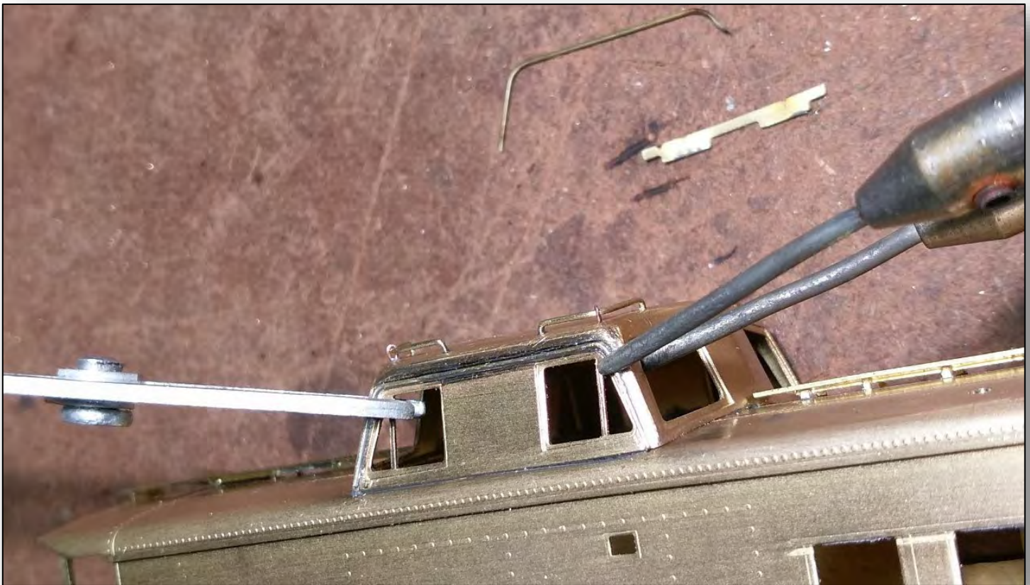
Method of attaching cupola rain gutter. Clamp is at left, tweezers are holding the part in place at right, ready to solder. Remnants of removed side window watershed and cupola rain gutter parts are visible above model.
