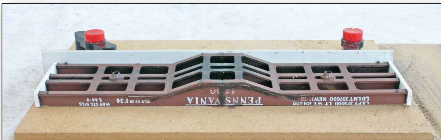
Figure 5 – Cuts made in stock Athearn frame so that frame bolsters are 9' from the end of the car.
