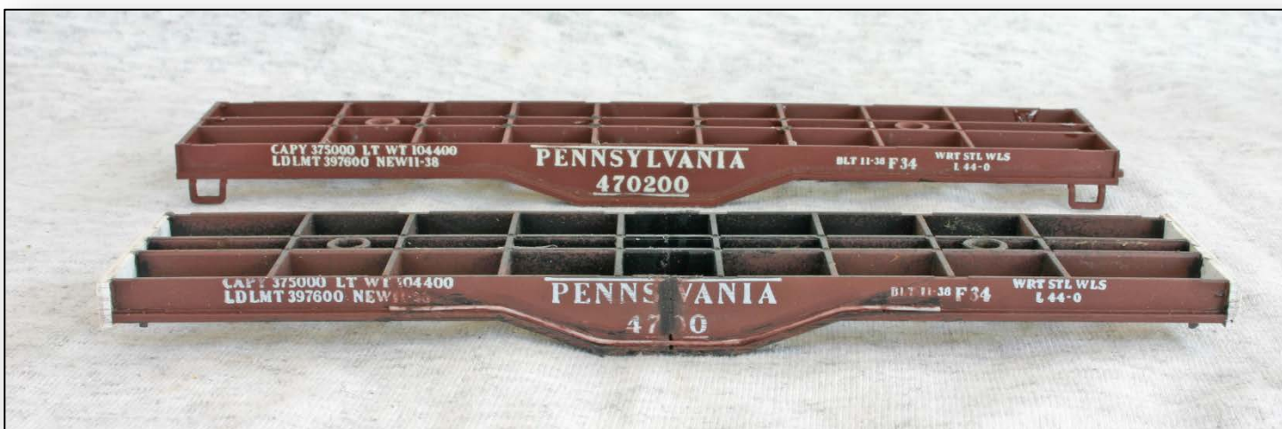
Figure 6 – Shortened frame and .02" rod applied to bottom of side sill compared to stock Athearn frame.
