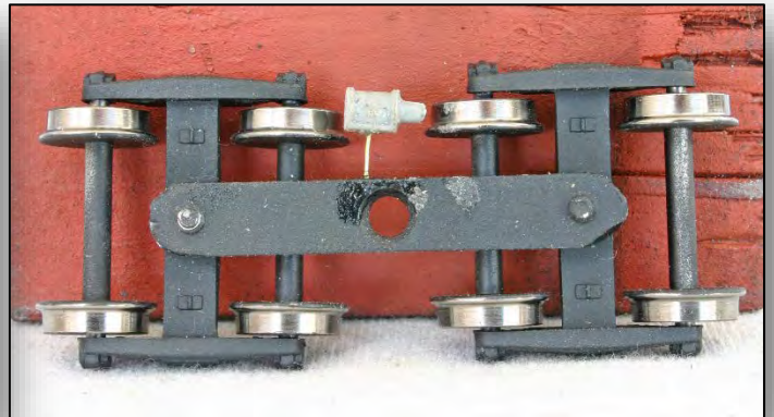
Figure 10 – Top view of trucks and span bolster. Note the inset of the center hole to fit over frame bolster.
