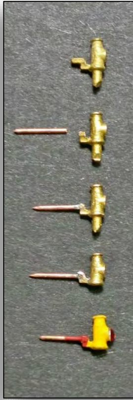
(Left) View showing cut lever, bracket and chain, new brakewheel and scribed end platform. (Center) Views of the modification steps for the marker lights and (right) the underside of the roof with the (red) wire insulation tubes glued in under corners for mounting marker lights.
