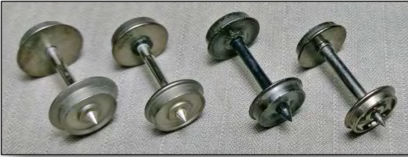
▲ For comparison, from left to right, Märklin 3-rail, TRIX, standard Kadee and ReBoxx narrow tread wheelsets. ► At left, N5C swing arm with coupler box and spring. At right swallow-tail NEM-362 couplers from bottom to top: Märklin European loop-style, TRIX Kadee-compatible and Kadee short shank size 17.
