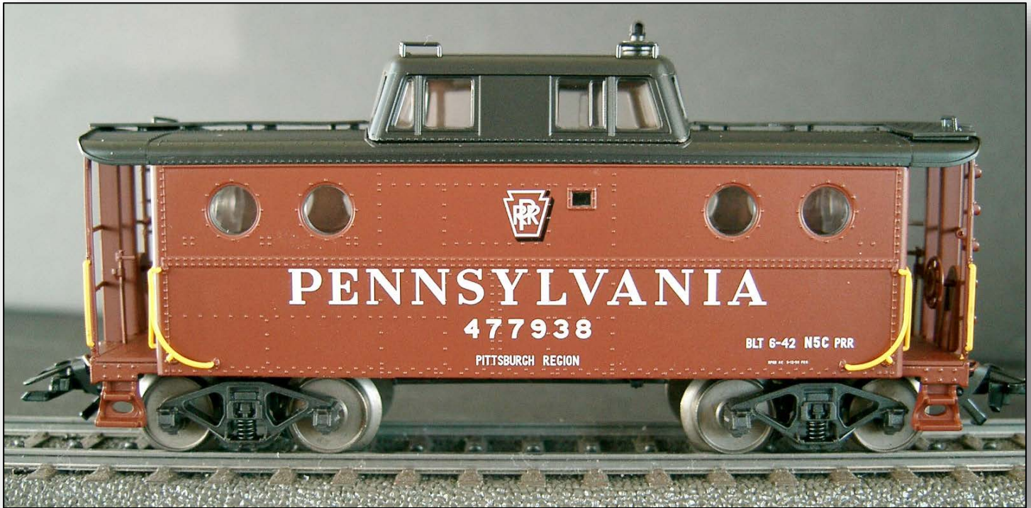
Märklin “3-rail” N5C Cabin Car shown on Märklin track. Rivets/buttons along center of ties form their equivalent of a third rail. Note couplers and wheels.
