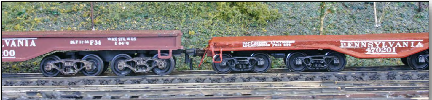
Figure 14 – Stirrup steps on model compared to Athearn model.
