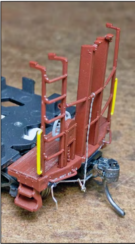
(Left) View showing cut lever, bracket and chain, new brakewheel and scribed end platform. (Center) Views of the modification steps for the marker lights and (right) the underside of the roof with the (red) wire insulation tubes glued in under corners for mounting marker lights.
