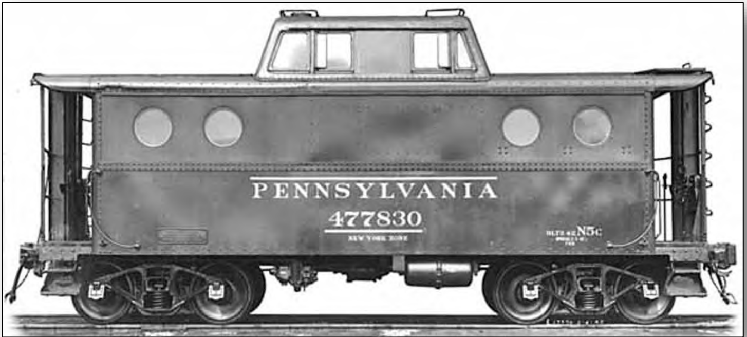
N5C #477830, assigned to the New York Zone, without Trainphone, 3/6/42. Note Equipment Trust plate at lower left and wind visors on cupola windows. (PRR)
