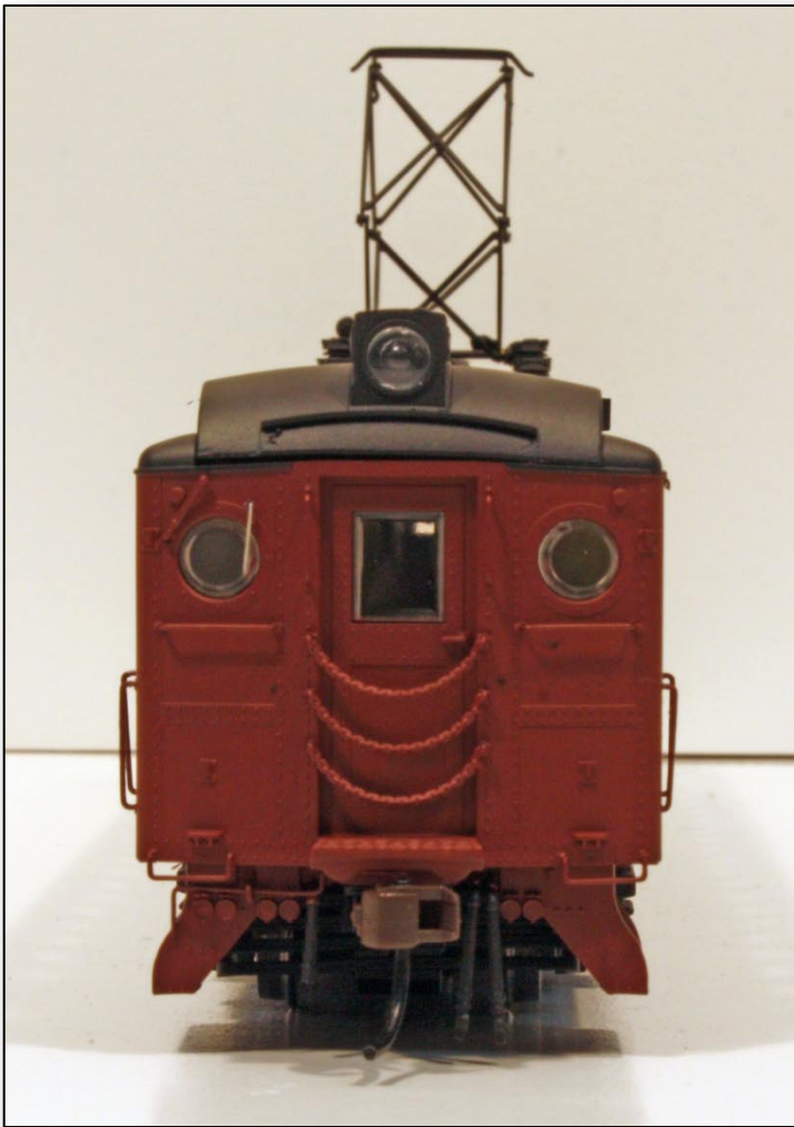
▲ Opposite ends of the powered car. The level of detail is amazing. Note the marker lights, windshield wipers, air whistle, chains, grab irons, cut levers, MU receptacles, hoses, and door latches. ▼ The pantograph details are exceptionally accurate.
