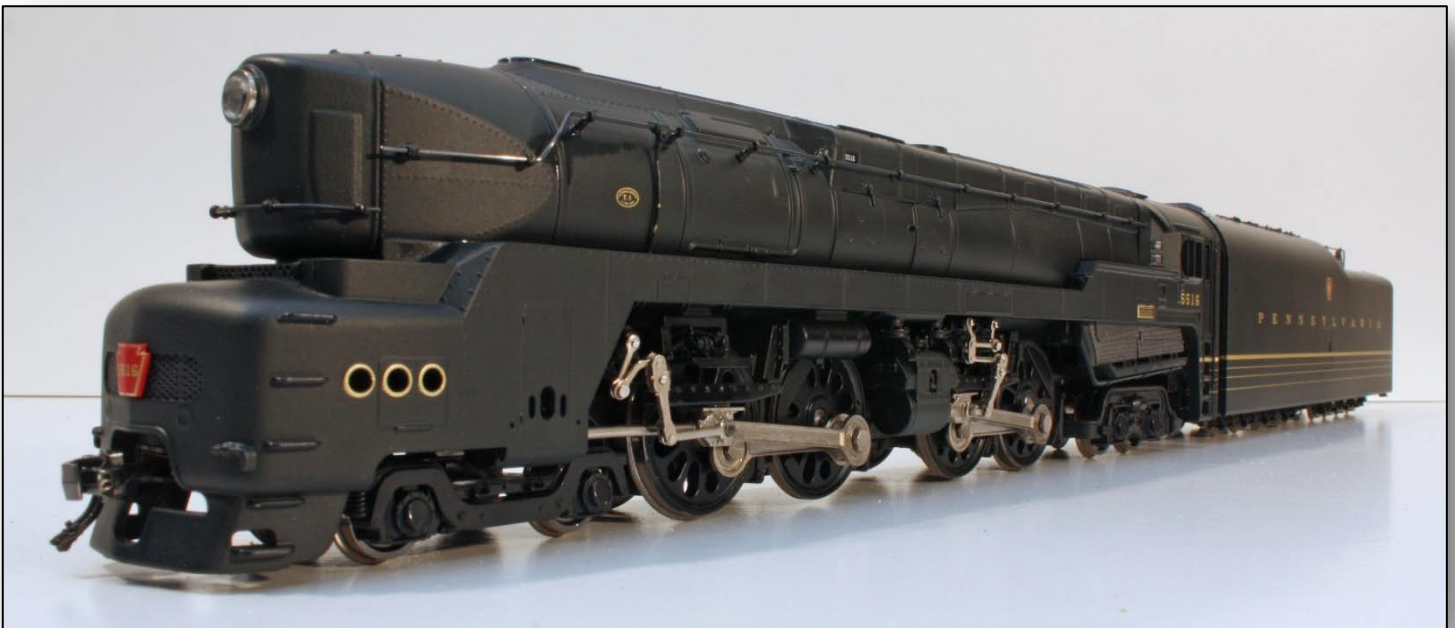
Wedge shot of left side. The portholes are a distinctive feature. Note the builder's plate on the side of the smokebox and free standing grabs on the pilot.
