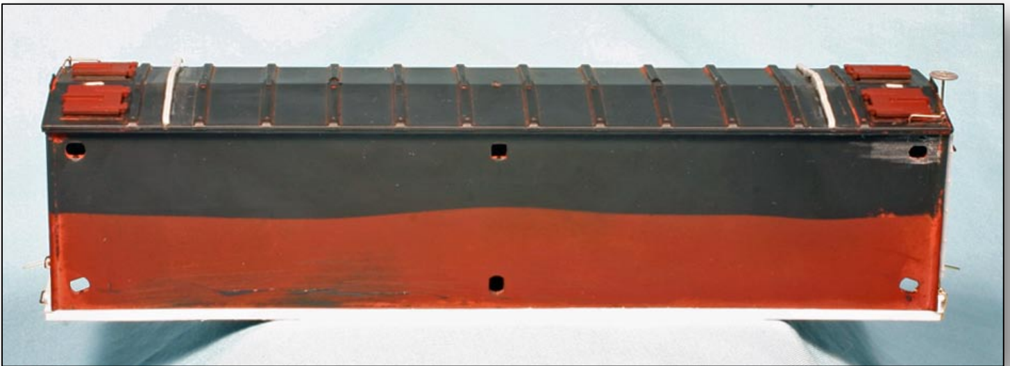
This photo shows the new side sill added to the bottom edge of the core. Additional details applied in later steps are also seen including end sills and hatch rests.
