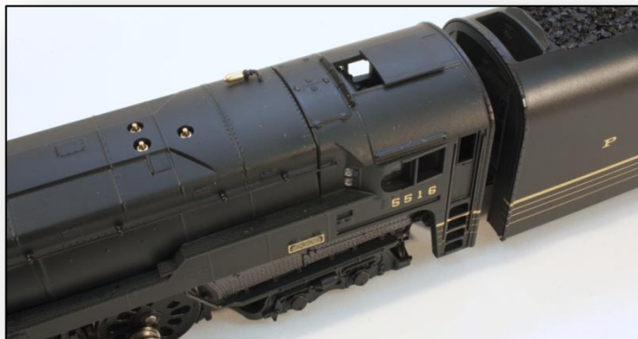
The cab detail includes a movable ventilation hatch. The whistle is closer to the cab on the "as-built" T1.
