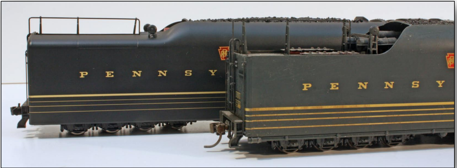
This shows the difference between the "As-built" tender to the rear and the modified tender in front. The modified tender has a different mounting for the Trainphone receiving coils and the rear cowling is cut away. Piping along the lower edge of the tender is exposed on both sides.
