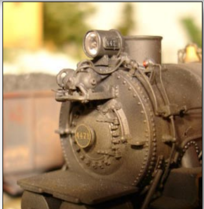
Close ups of the steam and electrical connections to the generator and electrical conduits to the marker lights.
