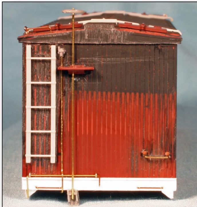
An end-on view of the B end of the 1922 built FGE reefer. Note the new end sill, corner gussets, wire grab irons, uncoupling lever, retainer valve and line and end ladder. New roof details such as grab irons and hatch rests are also visible.
