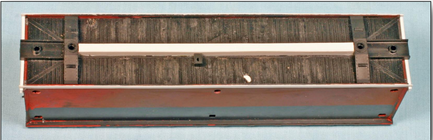
This photo shows the first steps in revising the underbody of the 1922 built FGE car. Most underbody details have been removed and the new center sill is in place.
