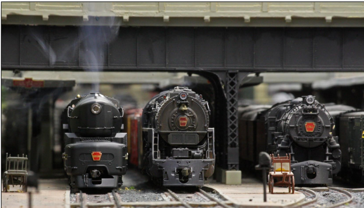
The smoke on the T1 is difficult to capture with a still camera, but is quite convincing when the smoke unit is warmed up. Smoke escapes from both stacks, is timed with the exhausts, and varies in volume with the load on the engine. The smoke volume can be adjusted at rest and moving with CVs and can be turned off temporarily with a function key or a switch inside the smokebox front.
