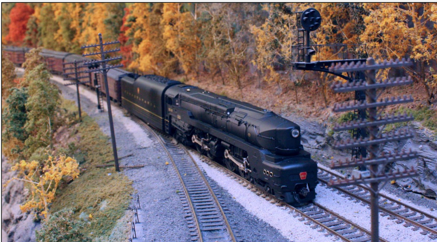
The smoke on the T1 is difficult to capture with a still camera, but is quite convincing when the smoke unit is warmed up. Smoke escapes from both stacks, is timed with the exhausts, and varies in volume with the load on the engine. The smoke volume can be adjusted at rest and moving with CVs and can be turned off temporarily with a function key or a switch inside the smokebox front.
