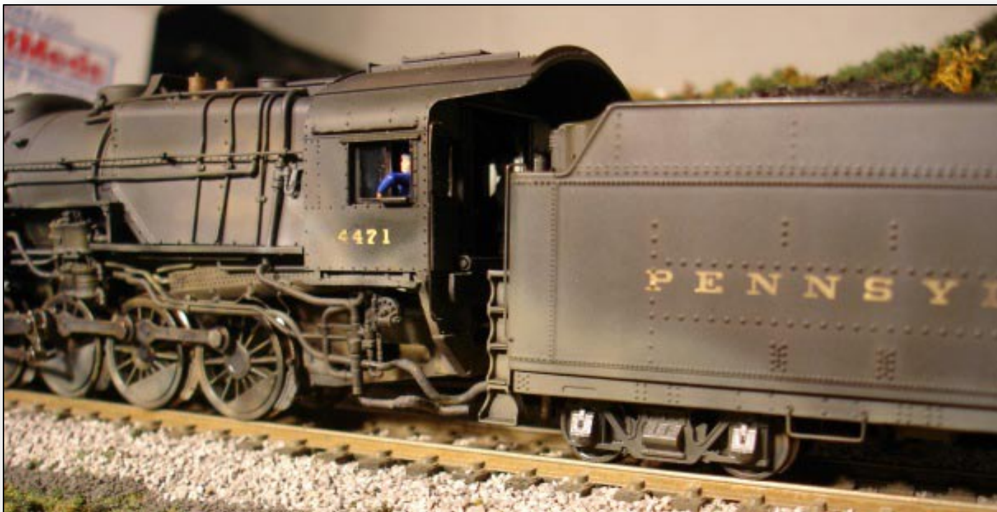
The completed engine-to-tender water hose connection.
