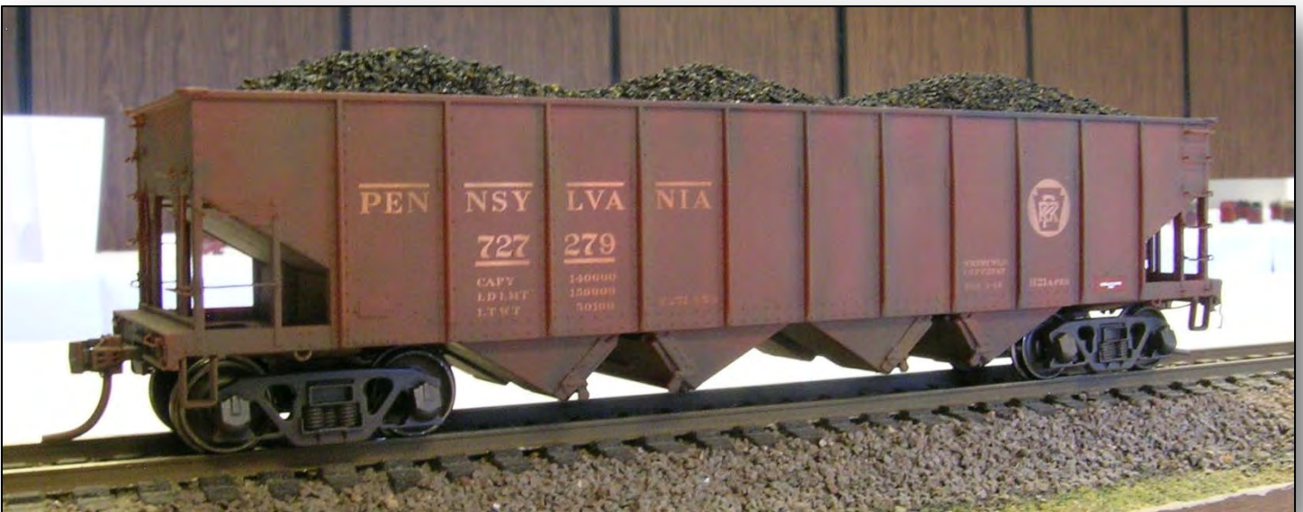
This HO H21A was a Bowser kit modified per the PRR PRO project discussions by Yank Yankolonis. This mid-fifties rendition of the car incorporates A-Line sheet lead weights in the center sill and a MOTRAK Models coal load.
