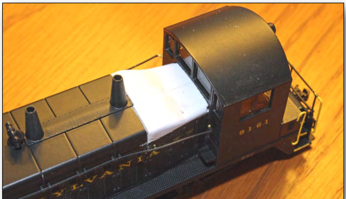
New hood piece fashioned from layers of styrene strip and sheet.
