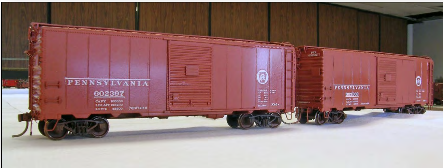
Tom Hayden kitbashed this pair of HO X43A boxcars starting with C&BT 12 panel boxcar kits. He scraped off the rivet details and added simulated weld seams. On 603062 he used fine copper wires. On 602397 he simply scribed lines in the plastic sides. Added details included Branchline roofwalks and end details, Kadee brake wheels and the cars were finished with Champ HB303N decals.
