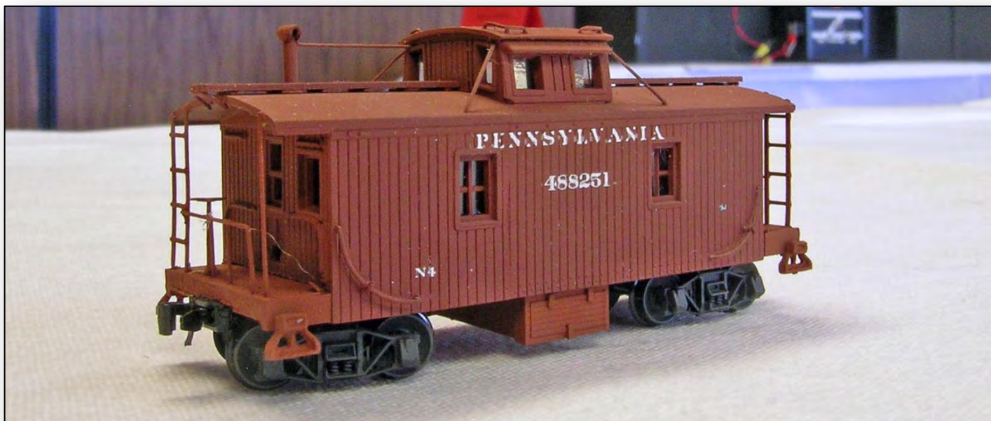
This N scale N4 cabin car was kitbashed by Claus Schlund from two Arnold cabooses. His model was built to represent the lone N4 prototype as it appeared in 1929.
