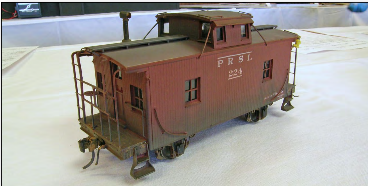
Buzz Burnley displayed an assortment of O scale Pennsylvania-Reading Seashore Lines equipment. This class ND cabin car was a brass model he painted with Floquil paints and added marker lights to represent a car used in the Atlantic City area in the early 1950's.
