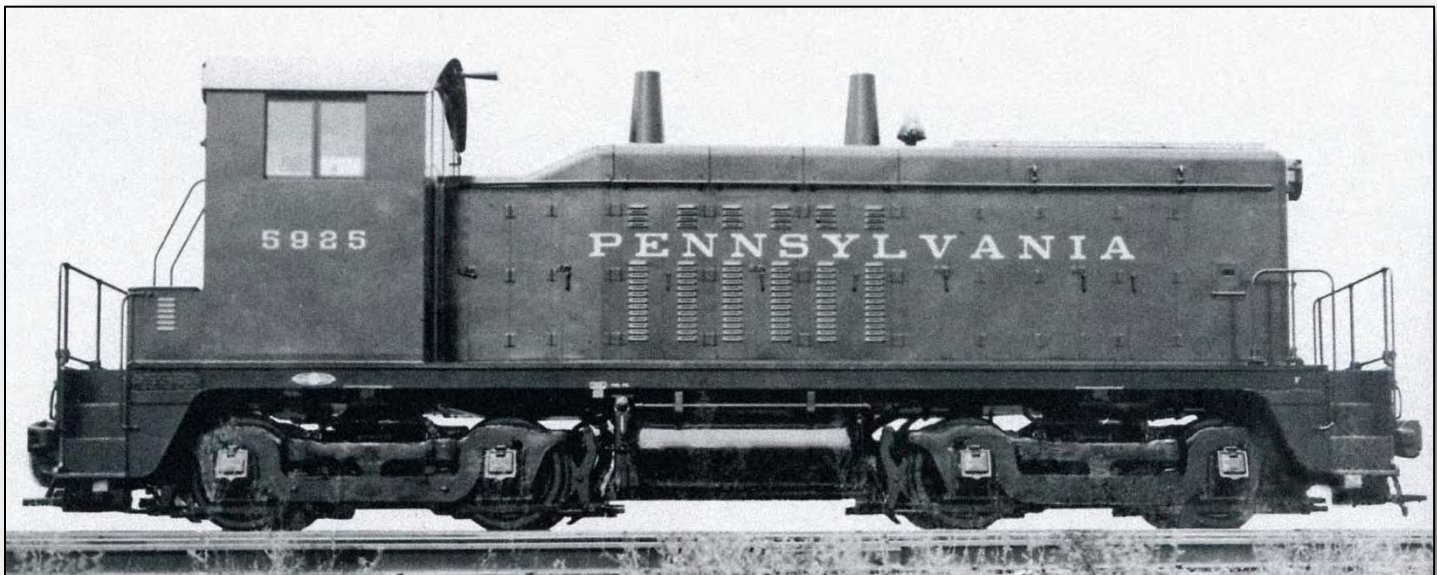
This builder's photo of NW2 #5925 displays the classic Phase IV details of most PRR units. It has the conical stacks, stepped hood, and side louvers with a gap for lettering. This was the road's fifth unit with a builder's date of October 1947.
