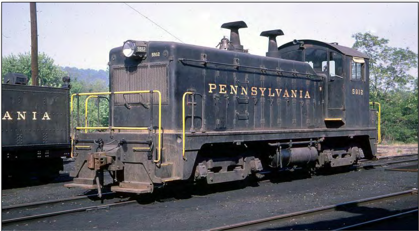
Here is the same unit renumbered to 5912 in Northumberland, Pa. on June 3, 1966. The straight stacks have been extended and capped with spark arrestors. Small marker lights have been added on the nose and a window shade has been added. Many of the handrails and edges of the stair treads are now yellow. (William D. Volkmer)
