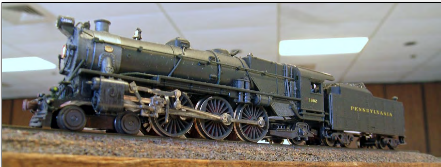
Doug Nelson's N scale K4s 3882 is a Minitrix model that has had many upgrades applied, including tender drive.
