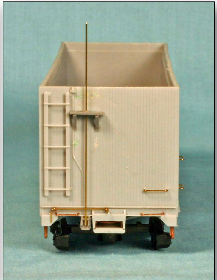
The A and B end of the car are detailed with grab irons, uncoupling levers, hand brake and other details.
