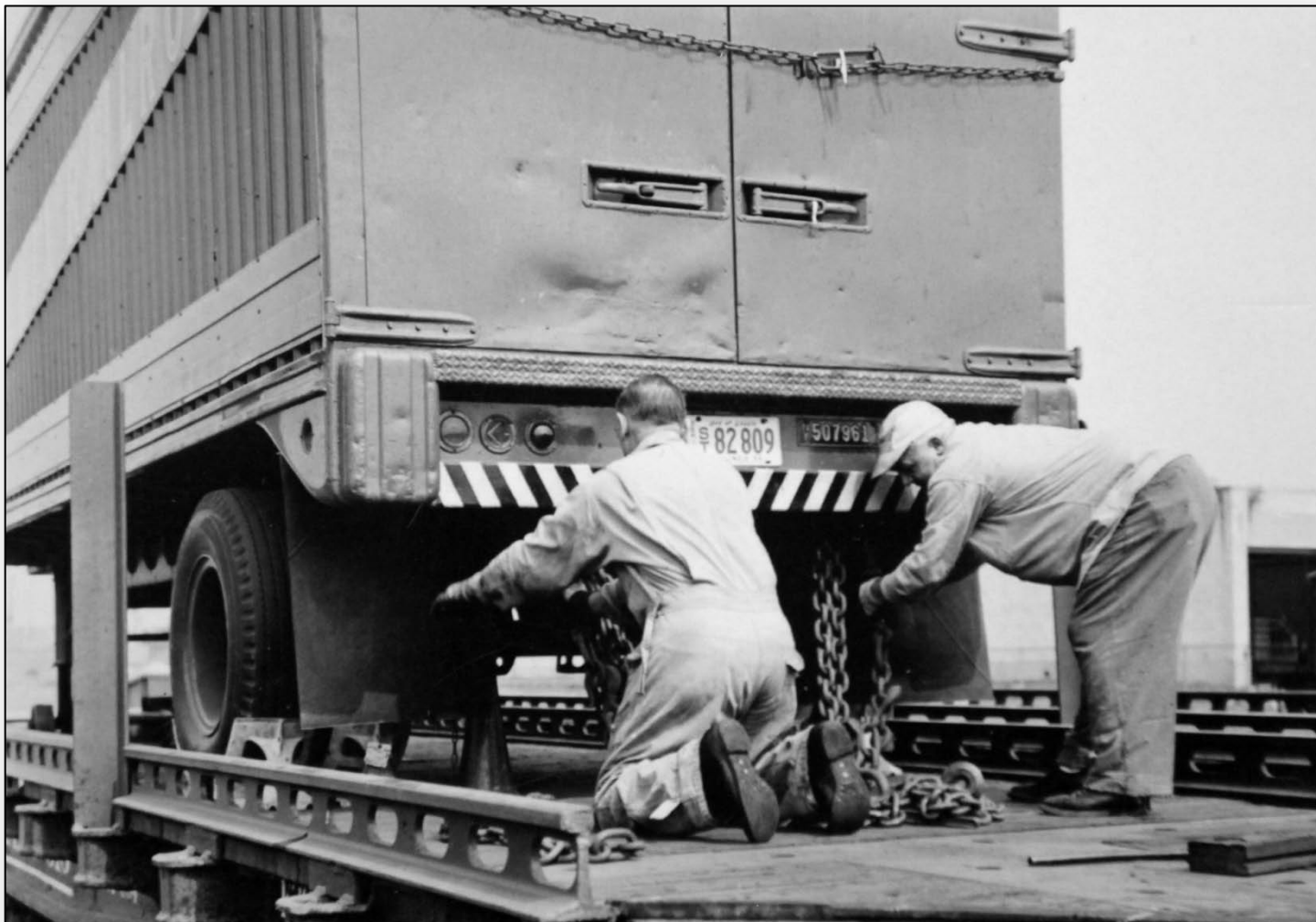
Note the heavy duty construction of rear bumper area with recessed panel for lights, the rubber dock bumpers, and striped bumper/ step. This trailer has recessed rear door latch handles. Some of these trailers were built with exposed rear door latch bars and handles. (Curt LaRue collection)
