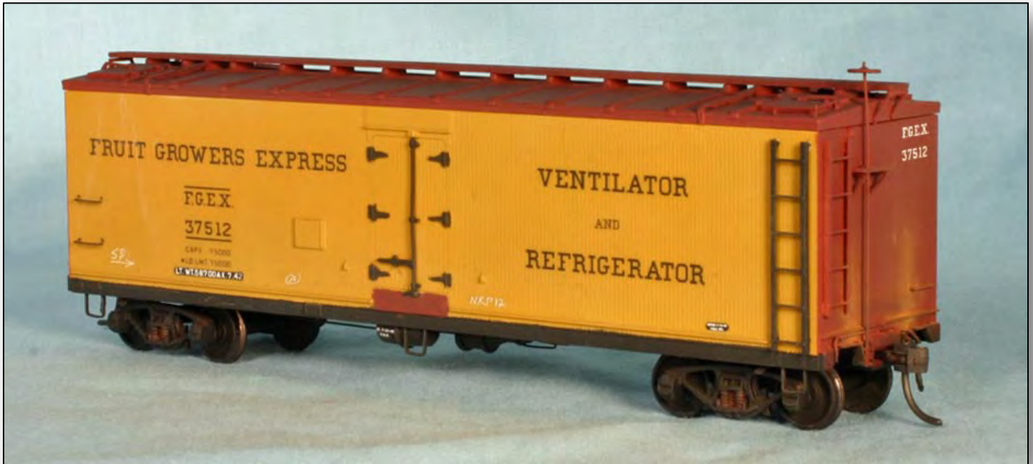
A side view of the model showing the lowered height as well as the removal of the plates from the side sill.
