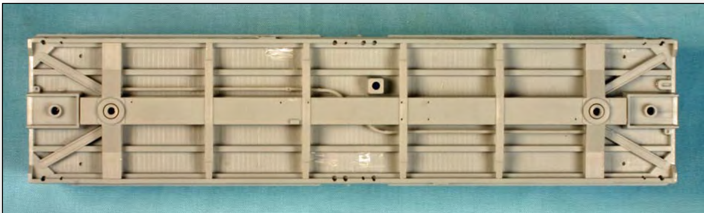
Photo of the bottom of the kit showing the underbody with the reservoir and AB valve mounting lugs removed and the air line, center sill and bolsters in place
