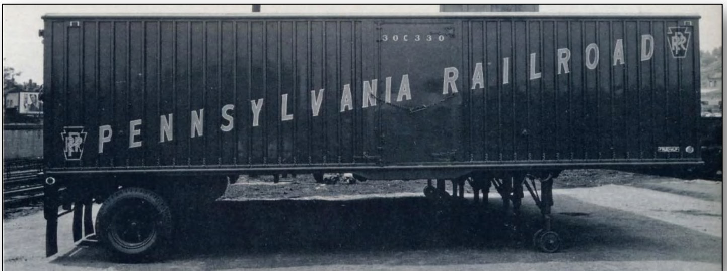
Side profile photo showing side details and lettering arrangement for trailer number 30C330. Note that trailer number is located near the top of side door. (Andrew J. Hart collection)
