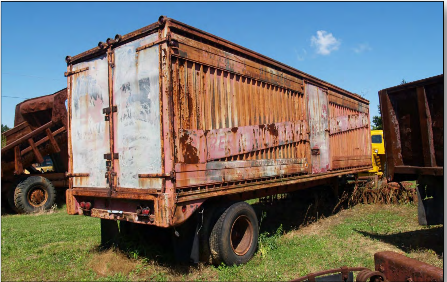
Three quarter view of rear and curbside of trailer. I believe that the rear door hinges and lights were later repairs made after taken from PRR service. Note the details of the rear bumper area with the recessed panel to protect rear lighting. (John Frantz)
