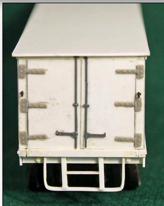
Rear view trailer showing location of rear door hinges and dual door bar latches, chain retainer eyelets, and details of rear step bumper. ►
