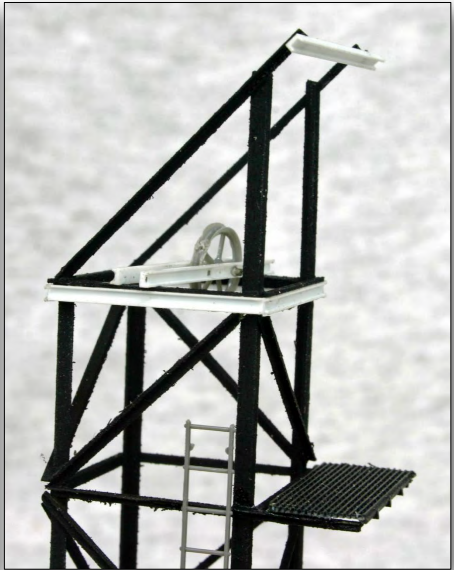
Details at top of tower. Note channels at top of highest section and at top of diagonals for chute sheaves.
