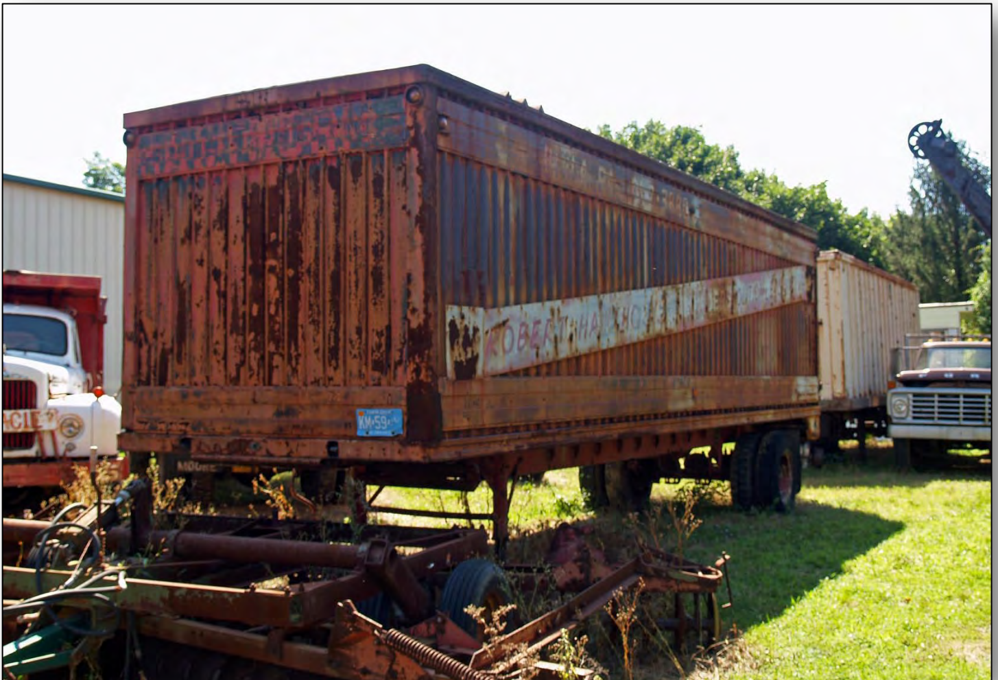
Three quarter view of nose and driver side of trailer showing scuff bands on nose of trailer. (John Frantz)
