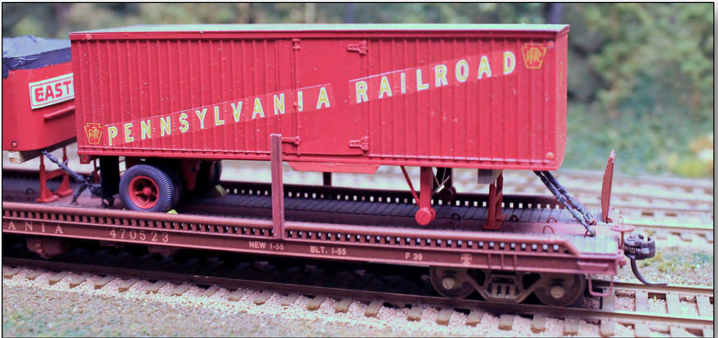
Model built earlier without keystone and lettering panels. Lettering applied directly over side ribs when the decals were fresh and conformed over ribs.
