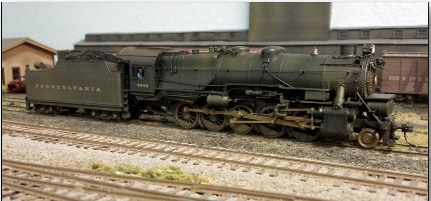
Number 4644 is another IISA with a big 210F82a tender, but it also has a right side air compressor. The model is a heavily modified Sunset engine with a PFM tender. It has the same added detail parts and improved drive train as 4324 and 4620. It has a TCS TI decoder.
