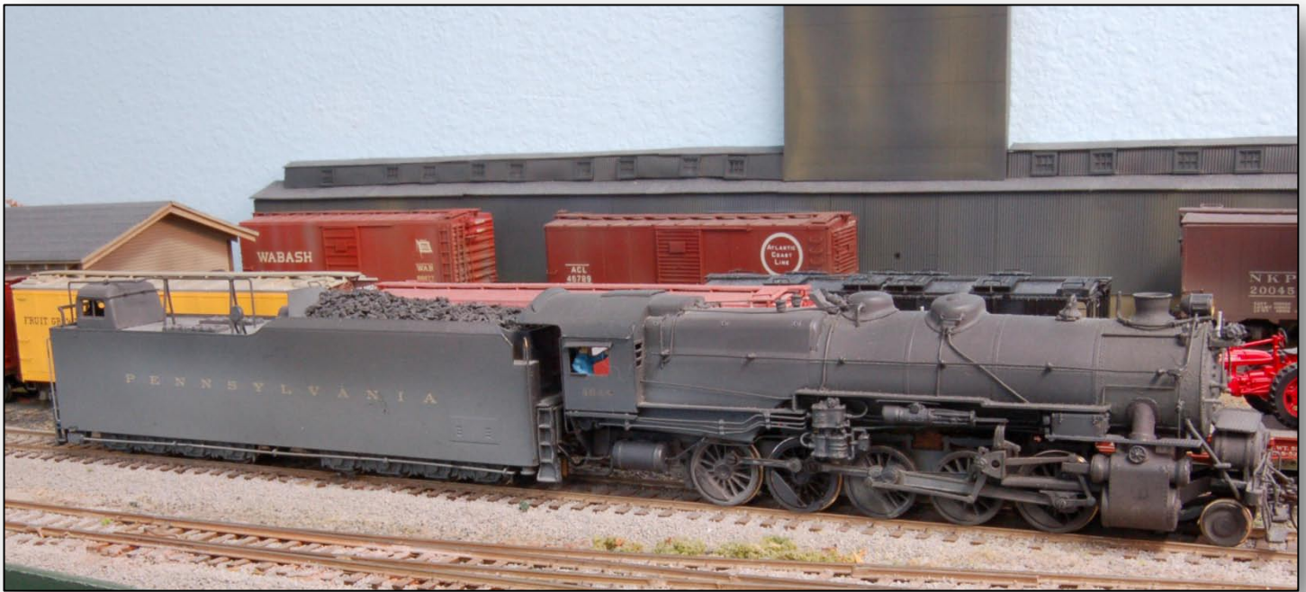
Number 4644 is another IISA with a big 210F82a tender, but it also has a right side air compressor. The model is a heavily modified Sunset engine with a PFM tender. It has the same added detail parts and improved drive train as 4324 and 4620. It has a TCS TI decoder.
