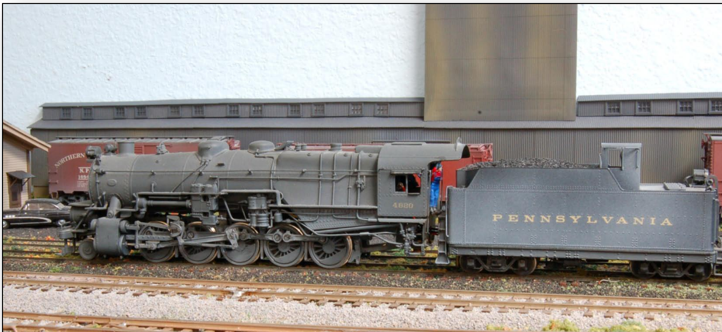
I1SA 4620 was later assigned to the Middle Division, but in October of 1953 it still called Northumberland home with "NEH," the symbol for Norry, painted on its pilot just as the prototype did. This is a PFM/United model with the left running board updated around the feedwater heater, bulls-eye markers from Cal-Scale, and a steel doghouse from Keystone Replicas. Also, a Precision Scale bell was installed. The drive train was updated with a Sagami motor and Precision Scale gearbox. It has a TCS TI decoder.
