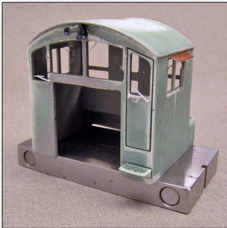
Modifications to the cab front include adding windshield wipers, horn bracket, sunshades and a door handle.
