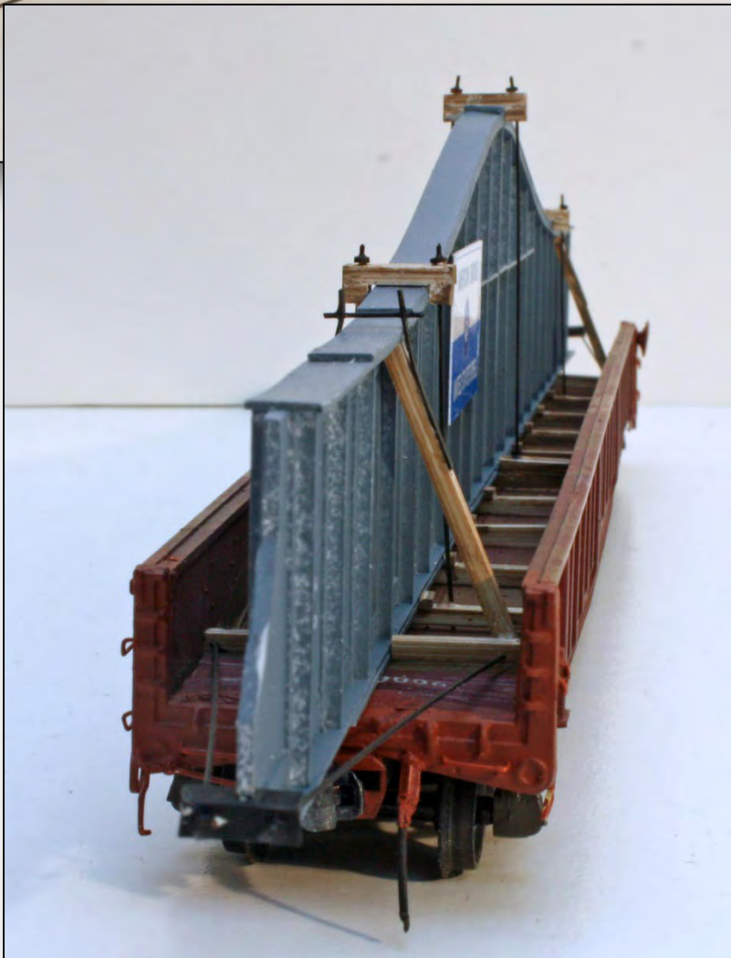
These views show the blocking on the load and the simulated nuts on the rods. The angled wood bracing has steel straps held by "bolts" at the top. The end view also shows I was a little light on the blue spray paint on this end. It's not noticeable on my layout, though.
