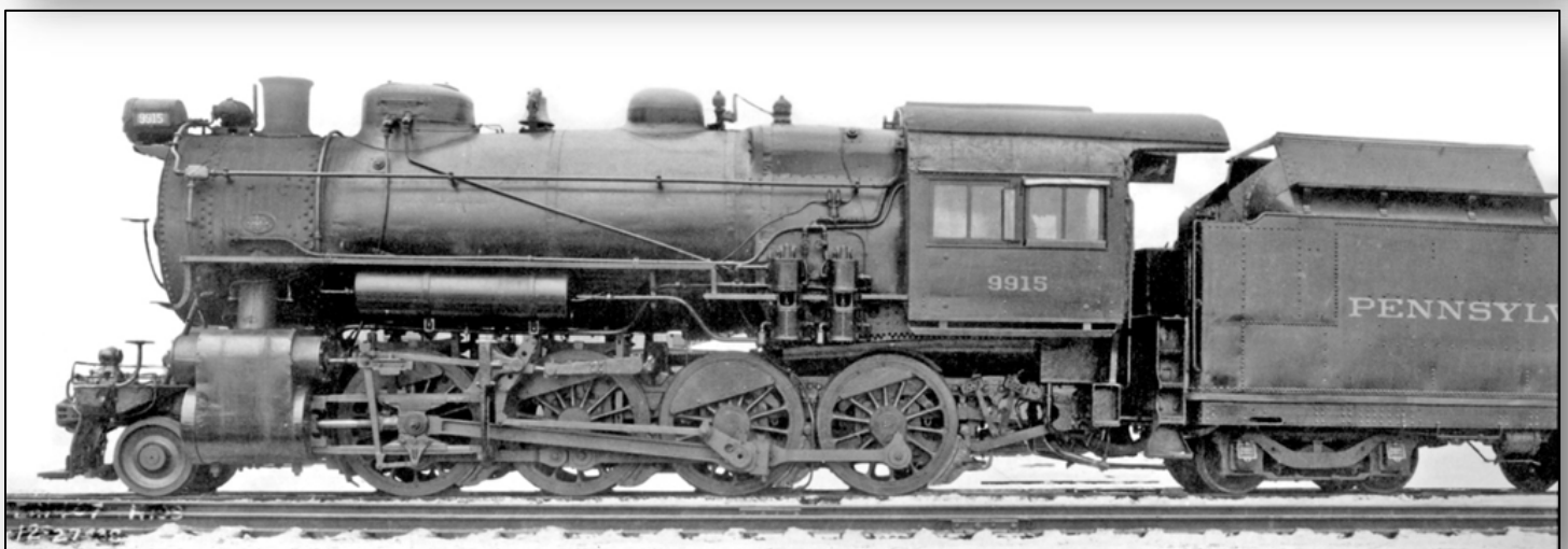
These two images were shot of Lines West H10s #9915 by PRR on December 27, 1938. These may have been taken for a booklet circulated at the 1939 New York World's Fair that showed equipment in operation on the PRR at that time. A few updated details are evident compared to the builder's photo – footboard pilot, claw-foot markers on the pilot and tender, electric headlight and generator mounted high, and an additional sand pipe behind the third driver. The standard narrow "toe-way" below the cab has been added. (PRR, Tim Garner collection)
