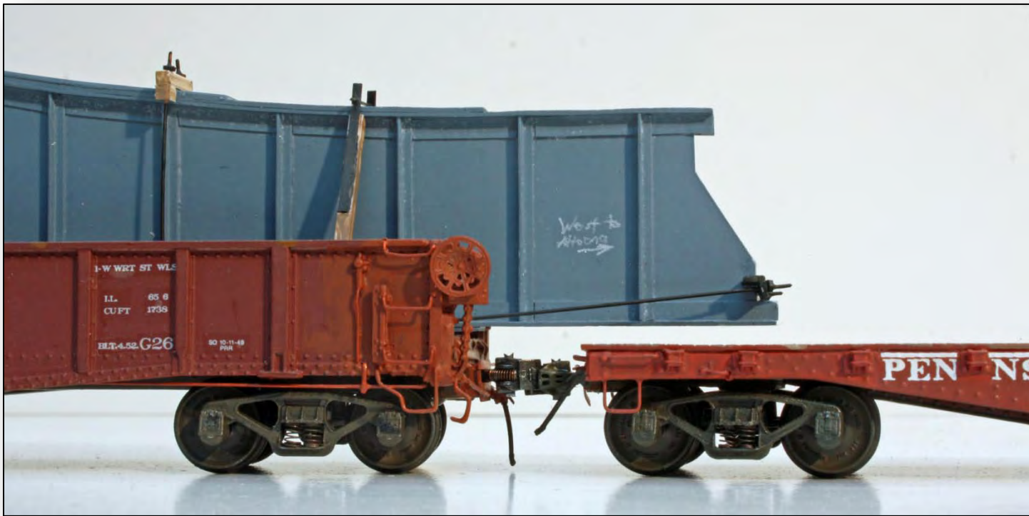
These images show how far the girder hangs over the FM idler flats. You can also see the chalk instructions written with an artist's pencil and the revised wire details on the G26 gondola.
