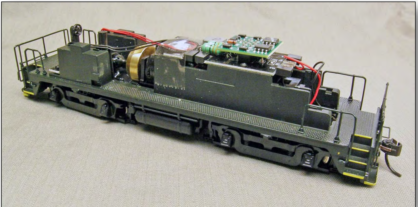
View of the drive unit with DCC decoder installed.
