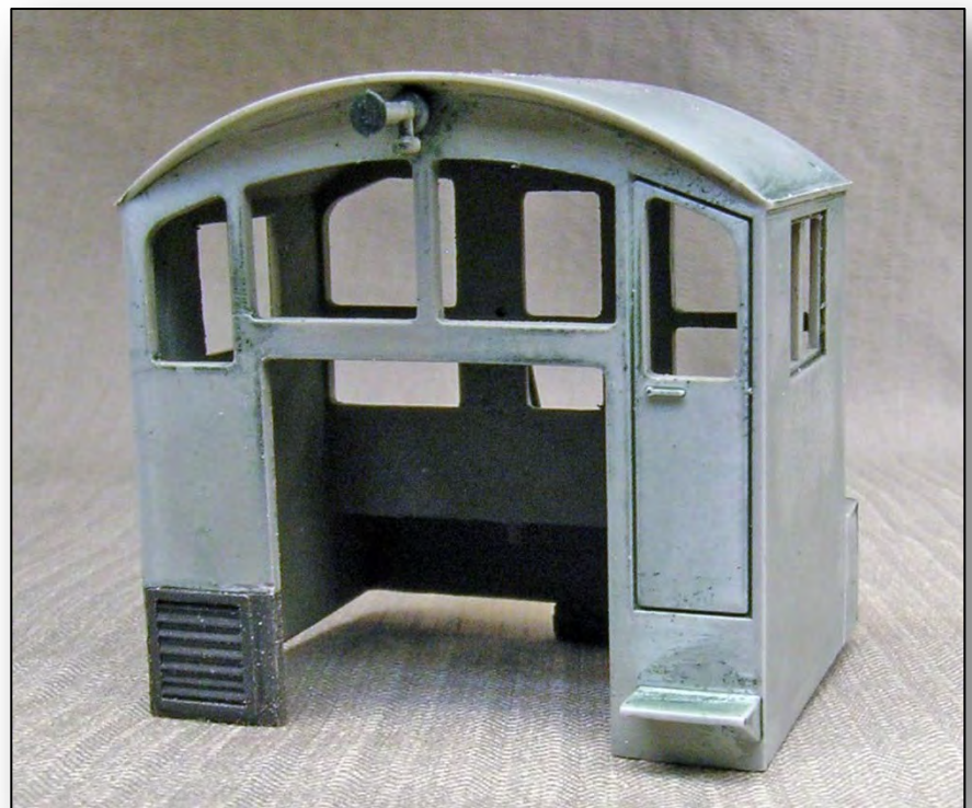
Modified Walthers cab to incorporate the post-1948 vent from an Athearn cab, here the black piece grafted into the cab front on the engineer's side just above the walkway.
