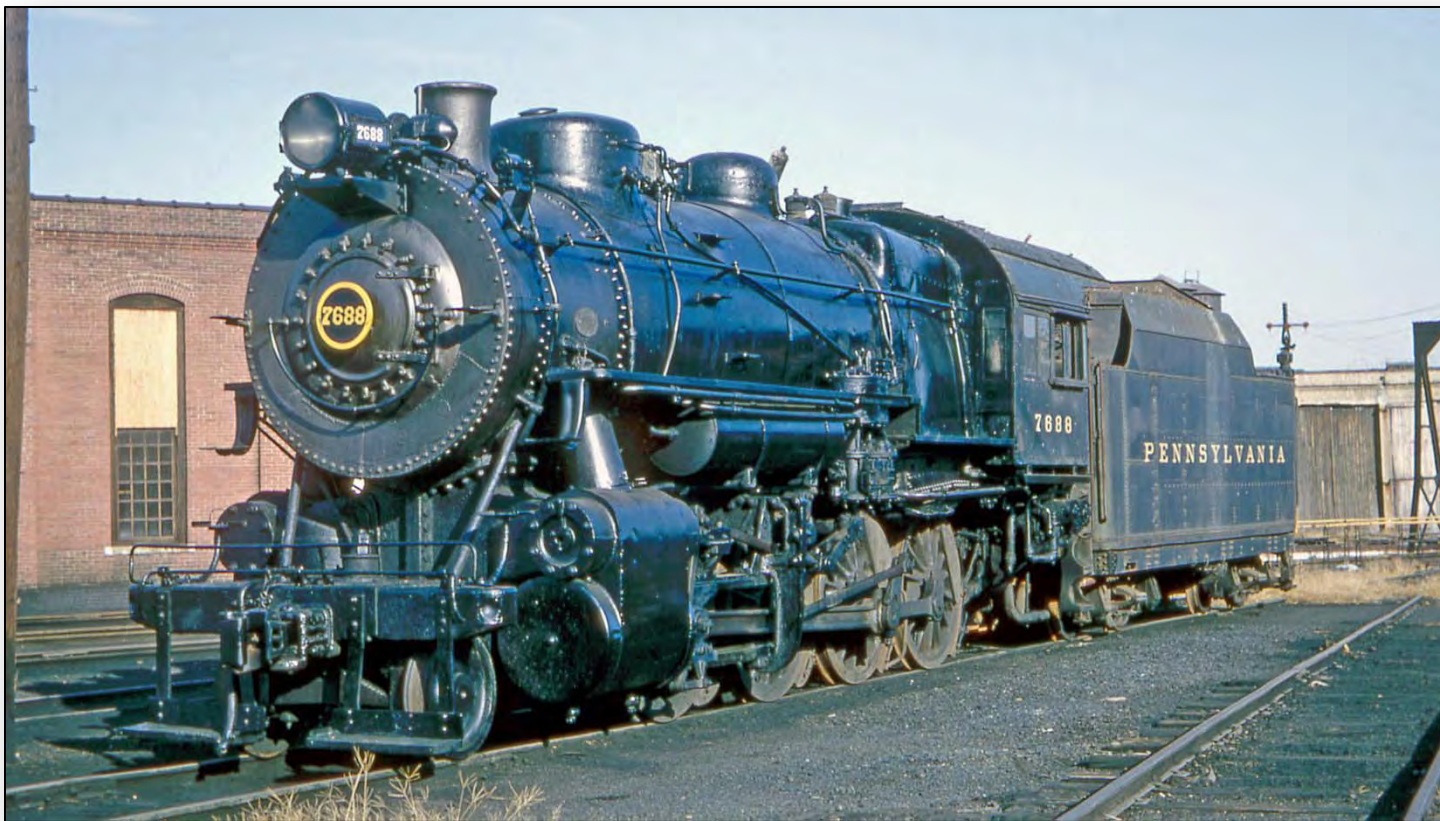
Preserved H10s #7688 is posing at the Northumberland Enginehouse on October 21, 1964. This engine is now on display at the Railroad Museum of Pennsylvania. The lower part of the smokebox front has had patches welded in at some point. (William D. Volkmer)
