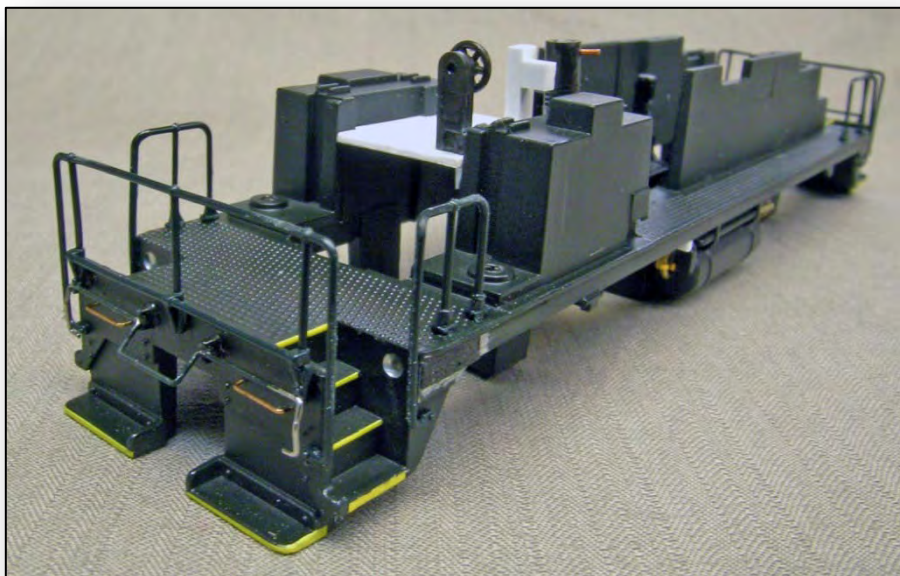
Rear view of the frame assembly shows the added pilot face grab irons, reconfigured cut lever, poling pocket recesses and (black) Trust plate added to the rear end of the sill. Also visible is the new cab floor with the added brake stand and relocated brake wheel.
