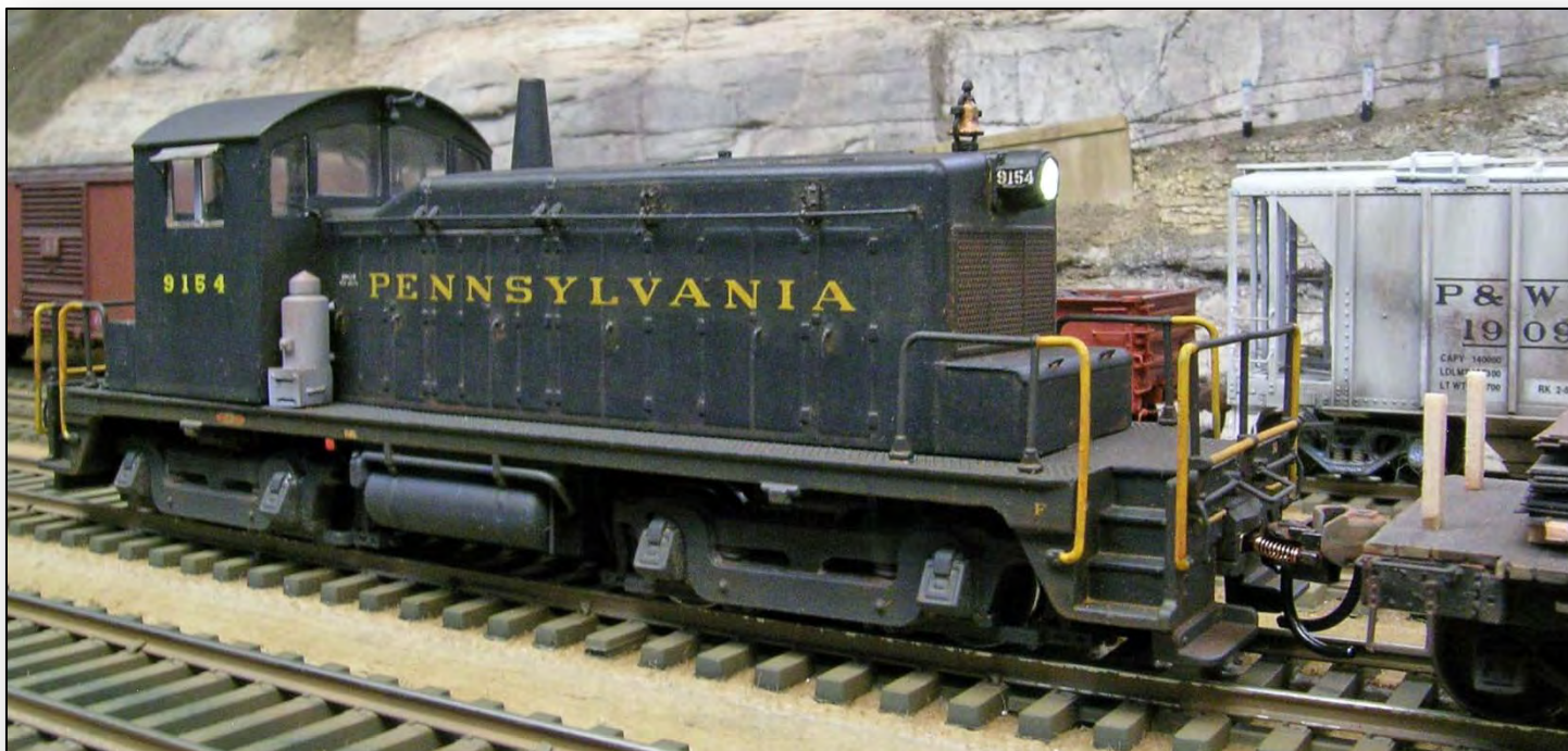
Completed unit showing block heater installed in front of cab on engineer's side.
