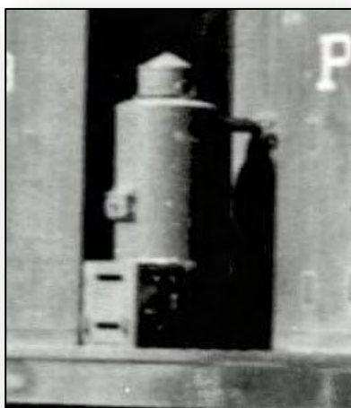
Left: detail view of #9143 shows block heater, painted body color by the time of this 1966 photo. Right: completed model block heater unit ready for painting.
