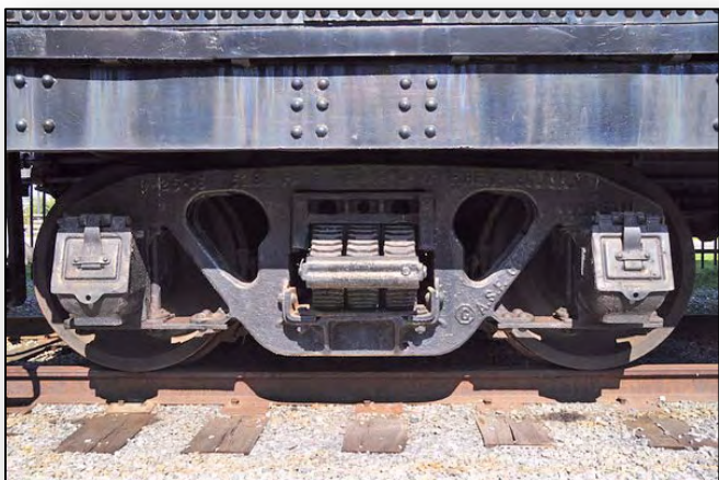
Figure 19. Close up photo of 2E-T2 trucks on tender for #7688. (Owen Thorne)
