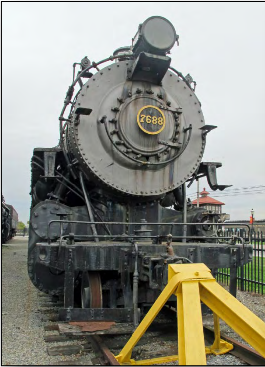
Figure 24. Photo of #7688 showing location of front marker lights. (Owen Thorne)
