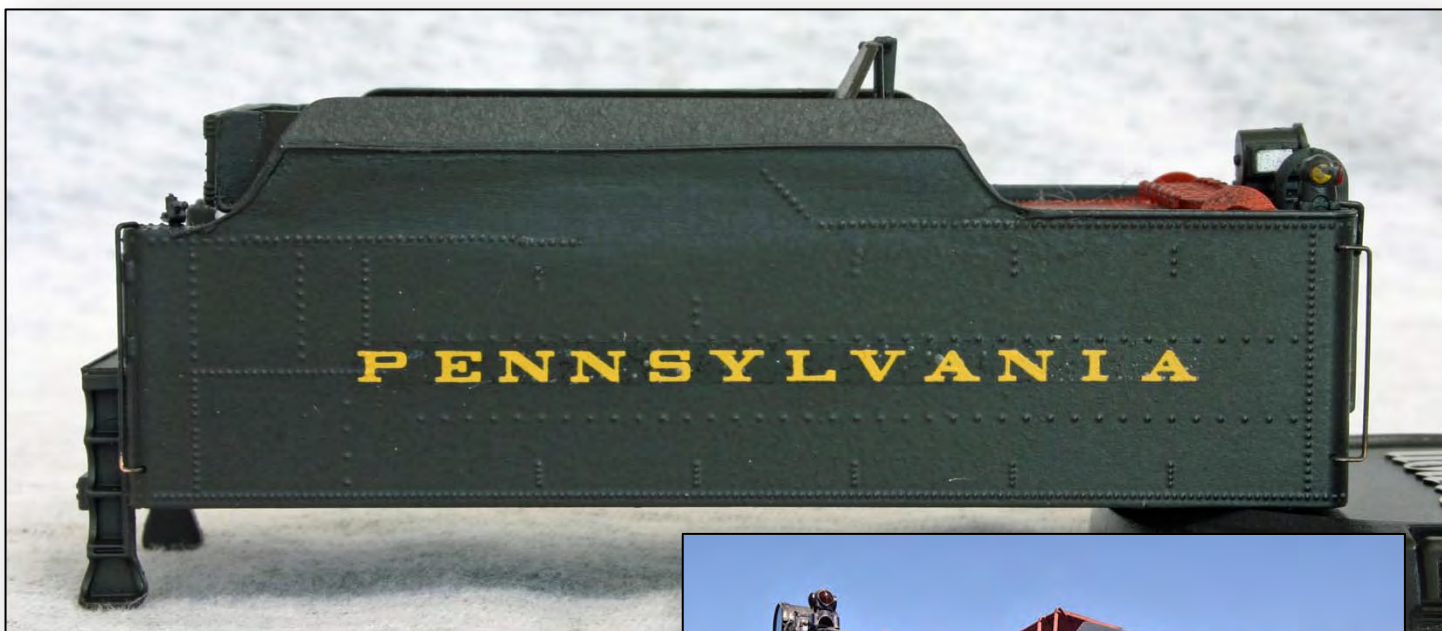
Figure 16. Model with new rivet lines (Micro-Mark rivet decals).
