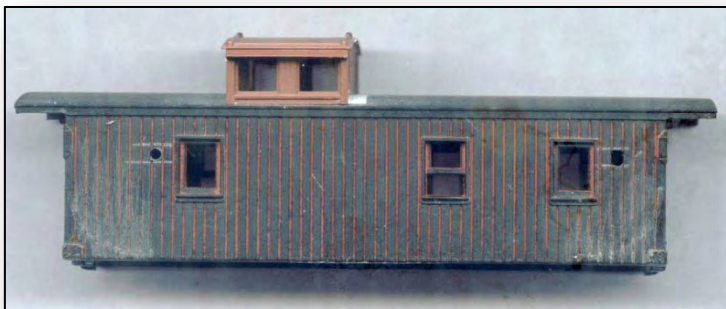
Figure 7. Body with holes for Watts marker lights.
