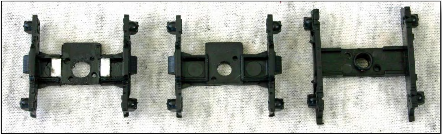
Figure 22. Underside of 2E-T2 truck, reinforced and filed to accept metal wipers of 2E-T1 truck (left), undersides of new 2E-T2 truck (middle) and 2E-T1 truck (right).
