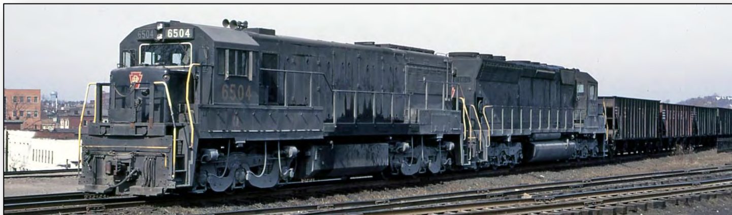
GF-25a (U25C) #6504 leads an EF-36 (EMD SD45) with a coal train through Wilkesburg, Pa. on February 21, 1969. Although this is technically Penn Central, the GE haulers were often paired with the big EMD's on mineral trains near the end of the PRR. (Ken Douglas, William D. Volkmer collection)
