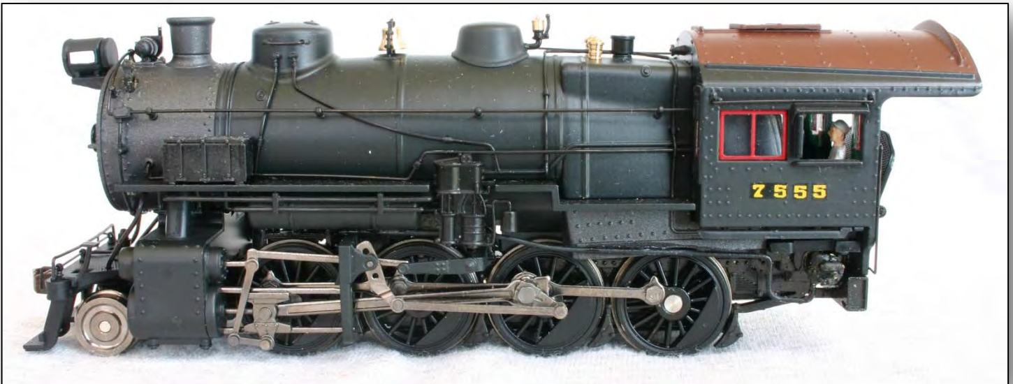
Figure 28. Fireman's side of #7555 showing Berkley stoker and signal box.
