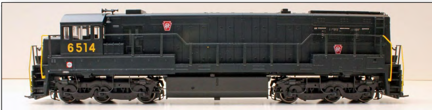
Rivarossi has captured PRR-specific details such as the train-control box behind the cab, the hump in the catwalk to the rear of the unit, and the placement of the horn and bell.
