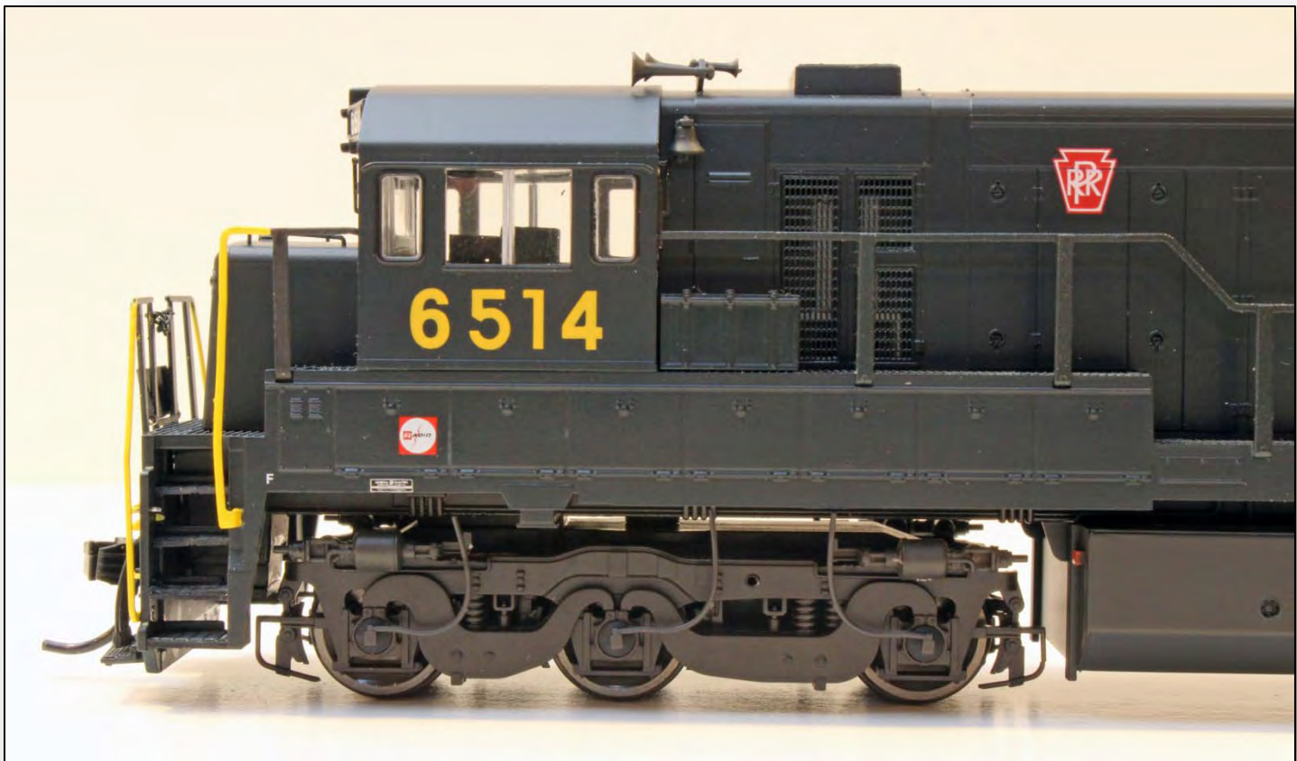
Rivarossi has captured early anti wheel-slip technology on the left side axle ends. Sand lines are included as it the unique PRR radio decal.
