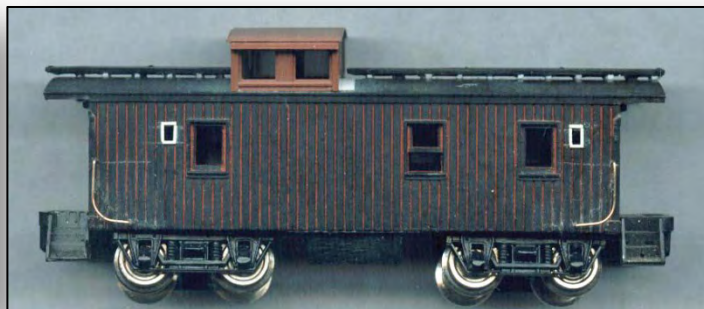
Figure 8. With Watts marker light openings framed with styrene.
