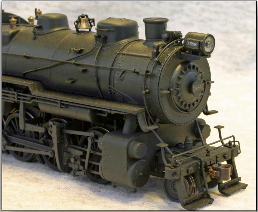
Figure 25. Model showing removal of pilot beam marker lights and addition of bull's eye marker lights on smokebox.
