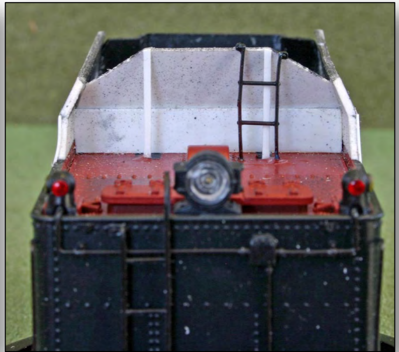
Figure 14. Rear view of tender with floor angle behind slope sheet, two vertical braces and ladder.
