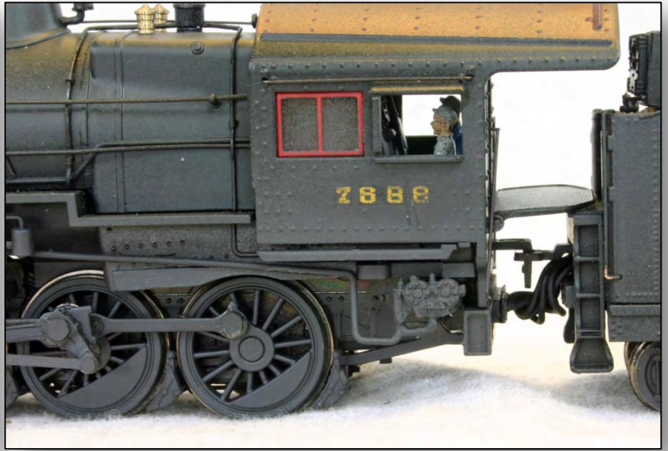
Figure 27. Fireman's side of #7688 with HT stoker and steam exhaust.
