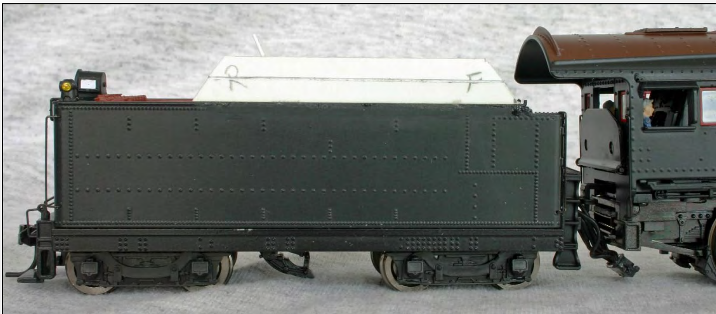
Figure 9. New side sheet extension attached to top chord of tender. Note: water scoop has not yet been removed and 2E-T1 trucks.
