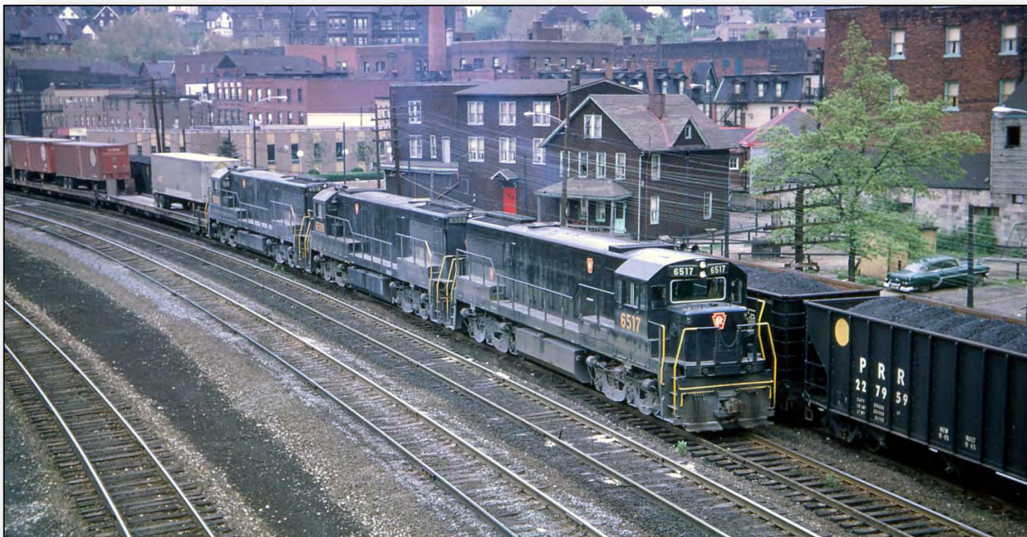
Here are GF-25a #6517, 6509, and 6510 on a TrucTrain in Wilmerding, Pa., east of Pittsburgh on May 21, 1966. Because of their low-speed lugging ability, they were more often found on coal and ore trains. (William D. Volkmer)
