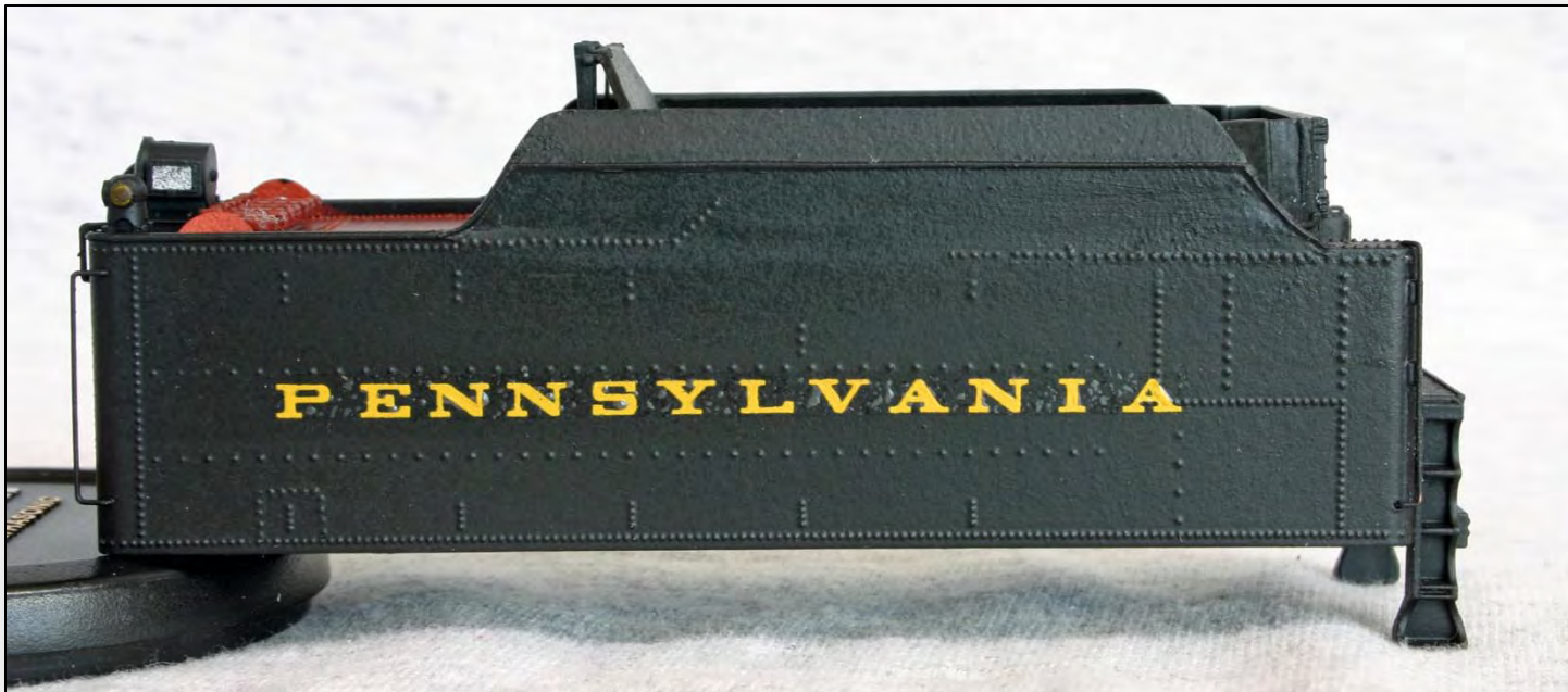
Figure 18. Model with new rivet lines, note patch (Micro-Mark rivet decals).
