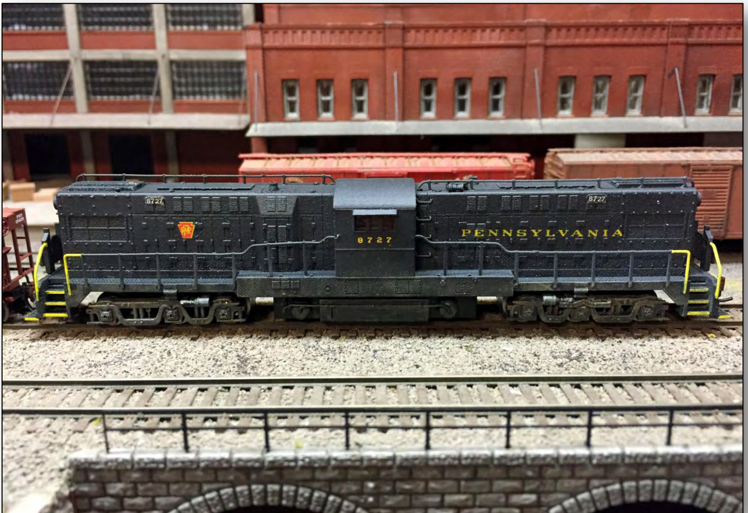
The completed shell with etched brass detail parts installed and ready for painting. The parts are all designed to snap in as replacement parts on an Atlas Alco Century 628 or 630.
